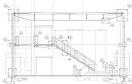
Section through the glass atrium with the stairs and the bridge hung from the steel structure above.
