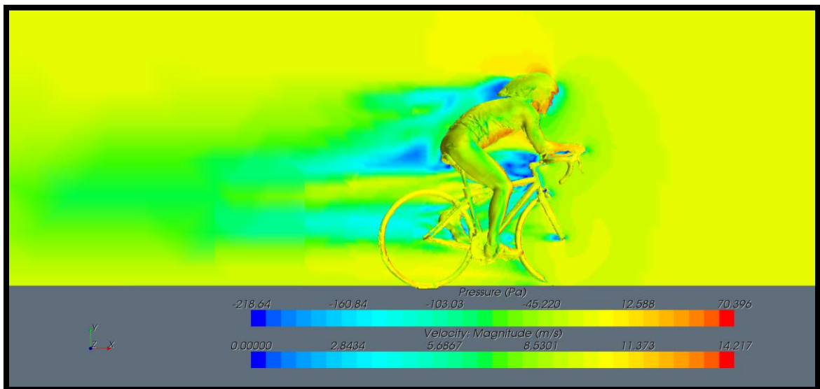
Figure 44 – Velocity and Pressure Plot of Symmetric Position at 12.5°
