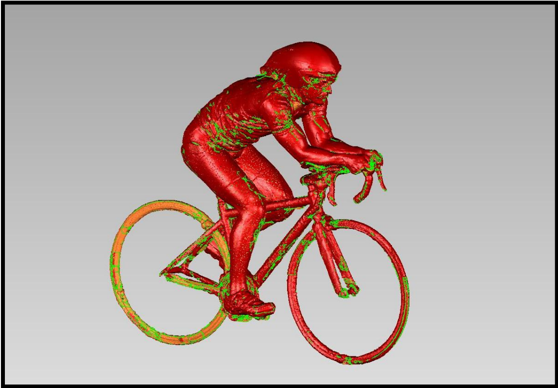
Figure 23 – Final Assembled Scan of Rider and Bicycle (After Significant Smoothing and Filling of Holes)
