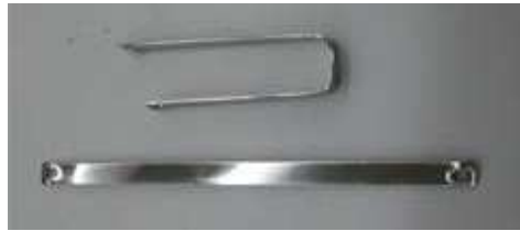
Figure 27 Design of stainless steel electrodes: Unbent (bottom) and Bent (top)
