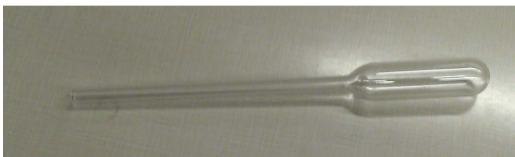
Figure 35: An Empty Ampoule with dimension 22mm outer diameter and 7mm length at the bottom with 19mm outer diameter at the top with thick wall tubing glass.
