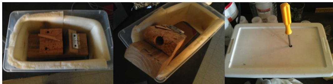
Figure 37: The Door Hinge Apparatus Used to Make Ampoule Breaking Safe
