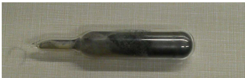
Figure 36: Sealed Ampoule after Step 1 of Intercalation
