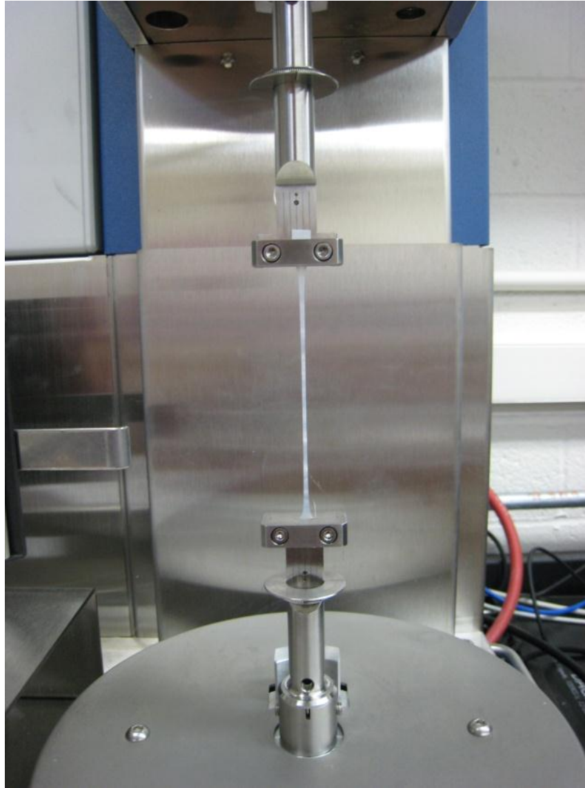
FIGURE 9 SEPARATOR SAMPLE OVEREXTENDED IN TRANSVERSE DIRECTION.
