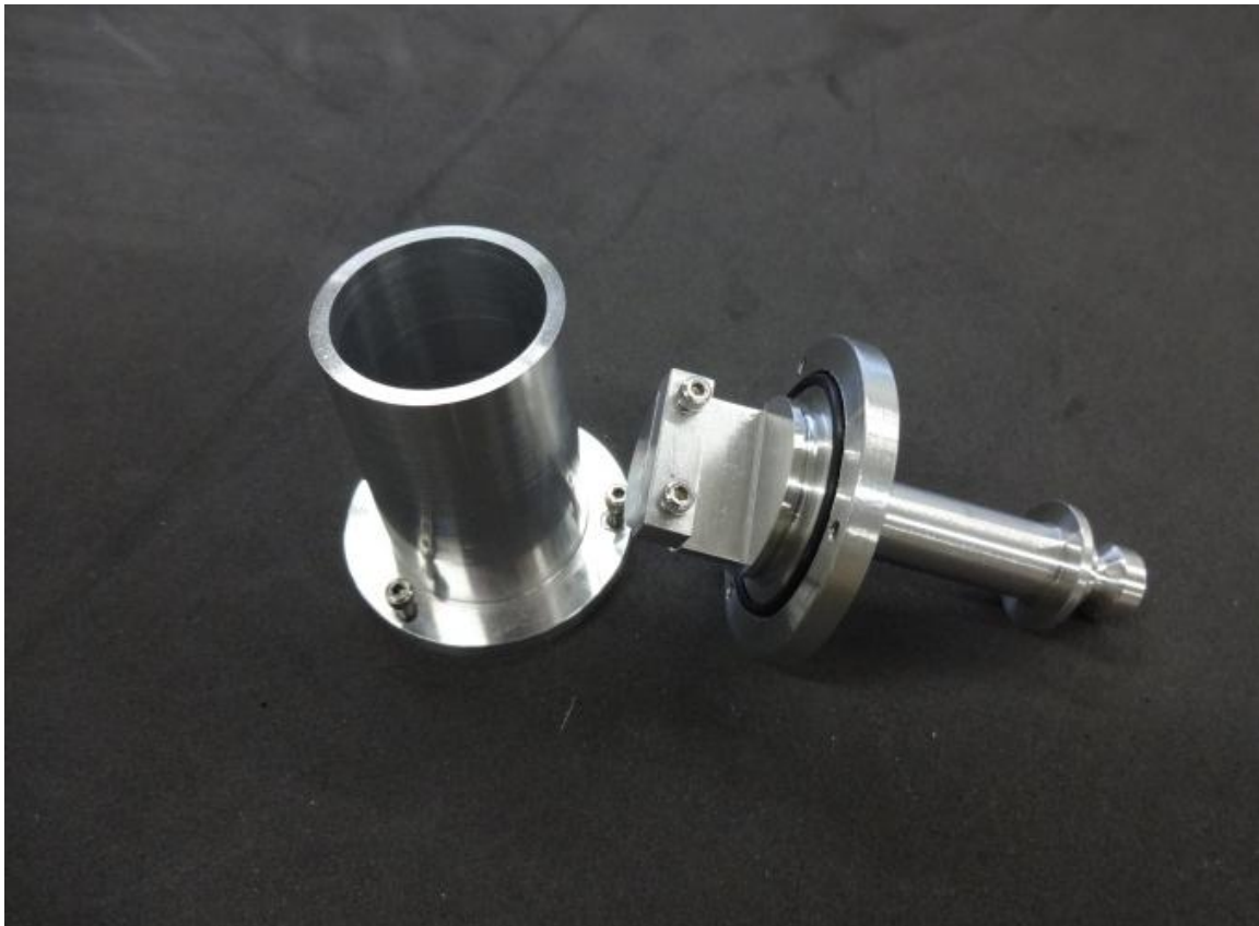
FIGURE 35 FABRICATED TENSILE TESTER WITH SATURATION CHAMBER
