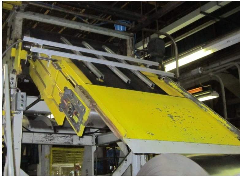
Figure 3-24: Prototype roller design mounted for testing
