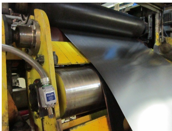
Figure 1-7: Metal sheet as it enters the pinch rolls
