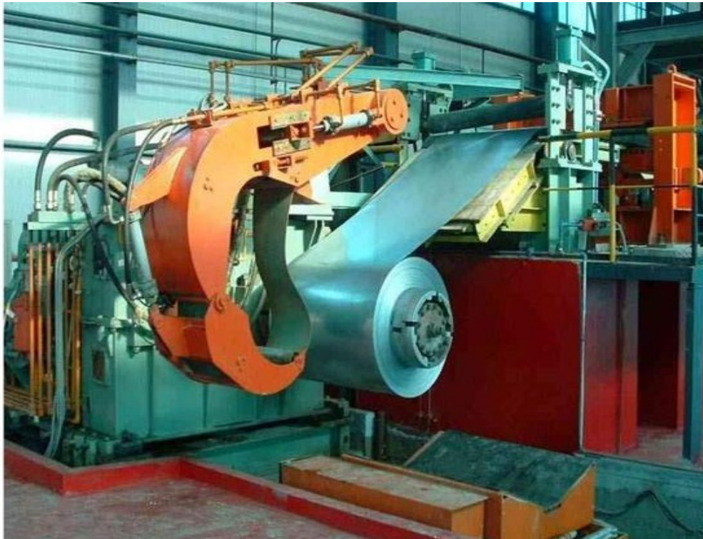
Figure 1-9: Coil line in-feed, Shanghai, China
