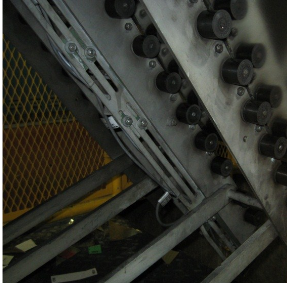
Figure 1-14: Under side of the rollers that sandwich the metal sheet
