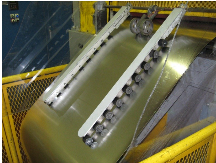
Figure 1-13: Roller bars mounted on the out-feed of the coil line servo feed machine
