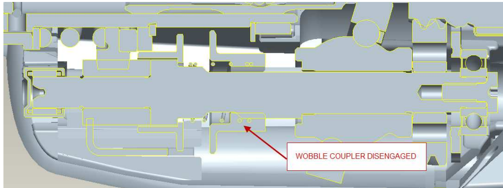
Figure 1-5 – Mechanism engaged in drill-only mode
