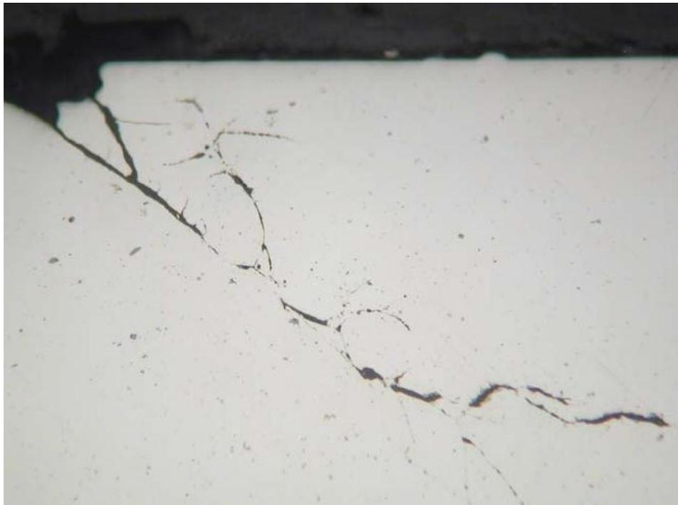
Figure 5.14: RCF-5-02, Crack location. Unetched (201X)
