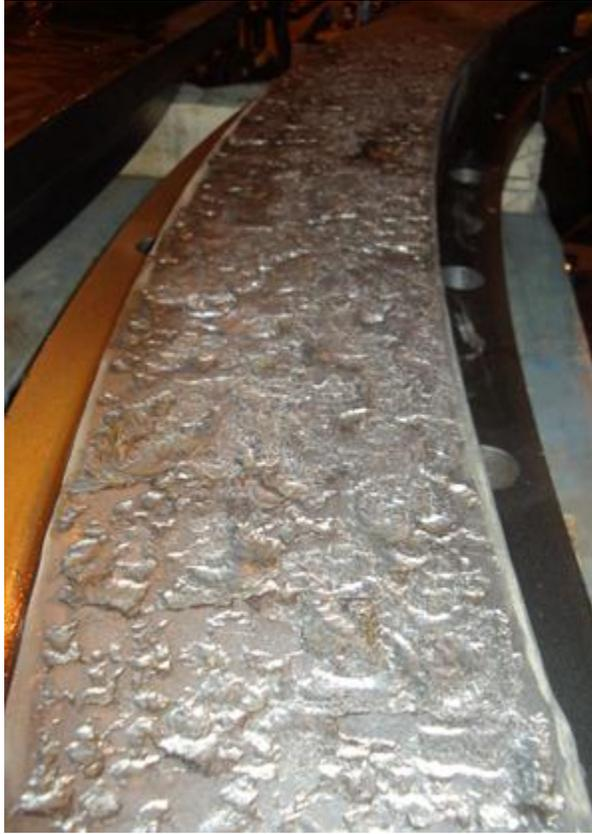
Figure 2.5: High carbon steel application failure mode
