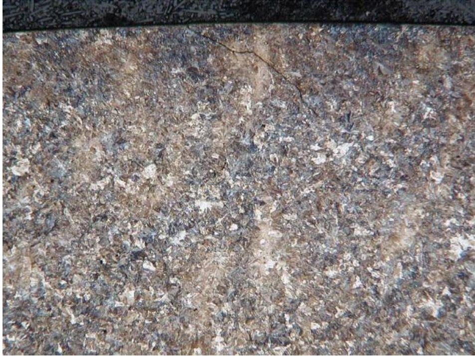
Figure 5.17: RCF-2-07, Microstructure. 2% Nital (50X)
