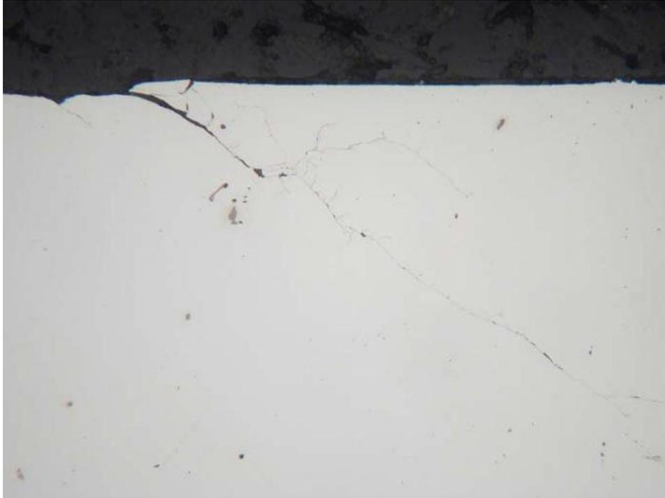
Figure 5.3: RCF-1-07, Crack location. Unetched (201X)
