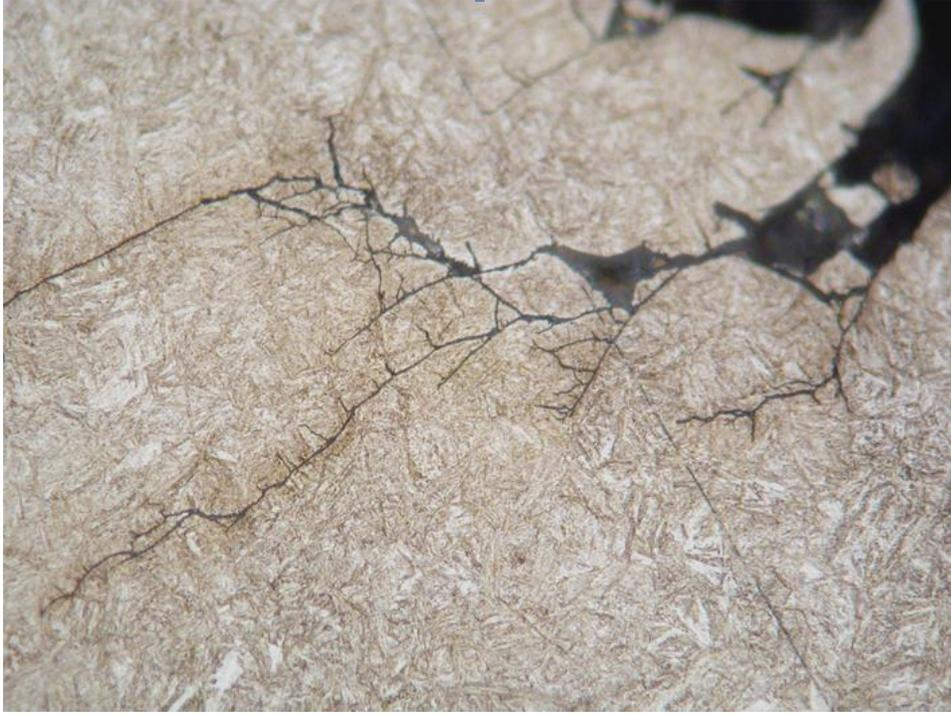
Figure 4.7: RCF-5-03-PRE Crack and Microstructure
