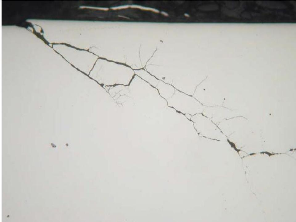
Figure 5.1: RCF-3-04, crack location. Unetched (201X)
