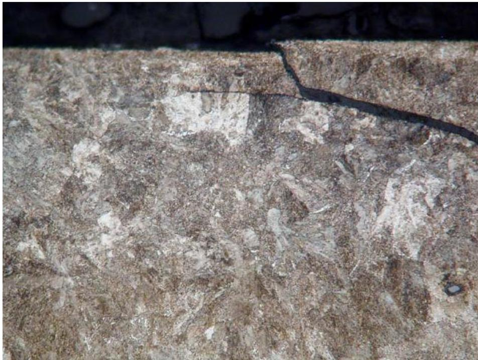
Figure 5.12: RCF-2-01, Near surface microstructure. 2% Nital (494X)
