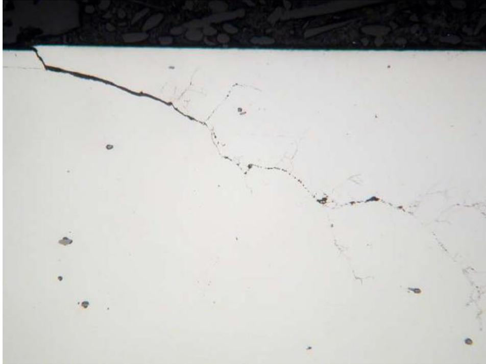
Figure 5.11: RCF-2-01, Crack location. Unetched (201X)
