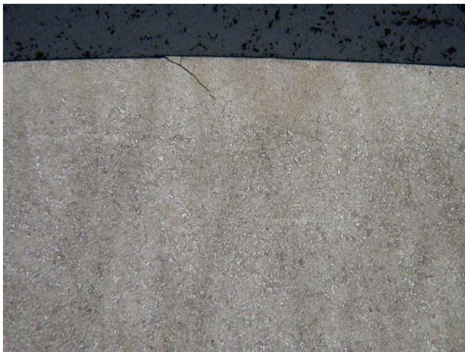
Figure 5.8: RCF-4-12, Microstructure. 2% Nital (50X)
