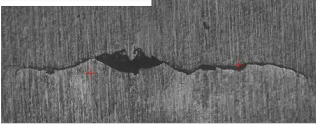
Figure 0.13: RCF-4-19, 10.2% Increased Contact Width, crack 1.2mm
