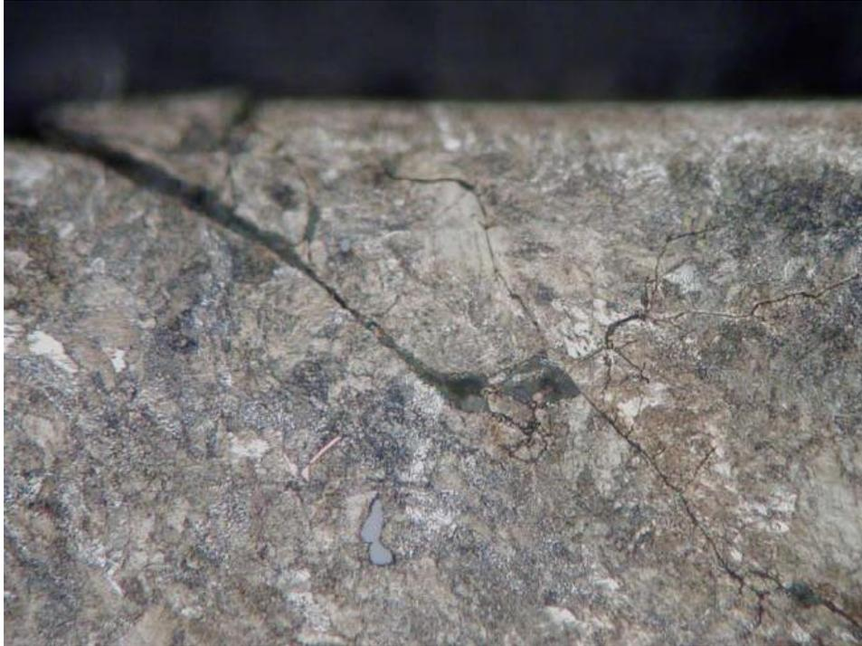
Figure 5.5: RCF-1-07, Transgranular crack. 2% Nital (494X)
