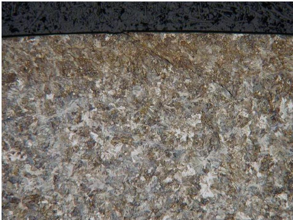
Figure 5.4: RCF-1-07, Microstructure. 2% Nital (50X)
