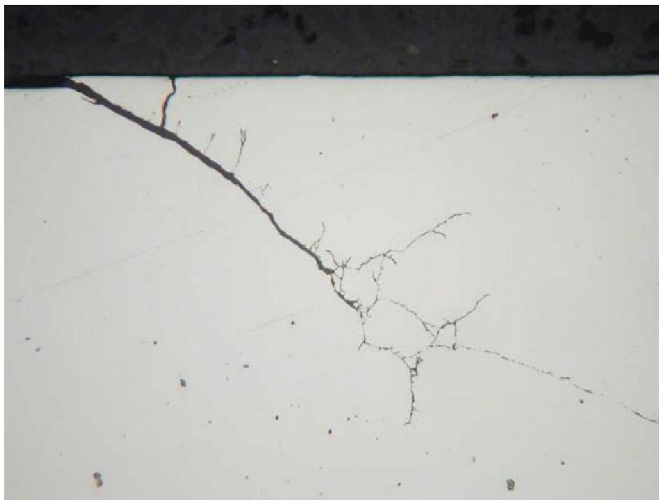
Figure 5.7: RCF-4-12, Crack location. Unetched (201X)
