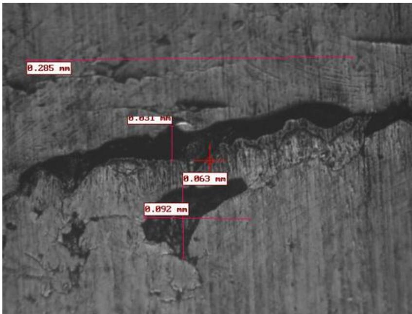
Figure 0.1: RCF-1-06, 30.8% Increased Contact Width, crack 2.1mm
