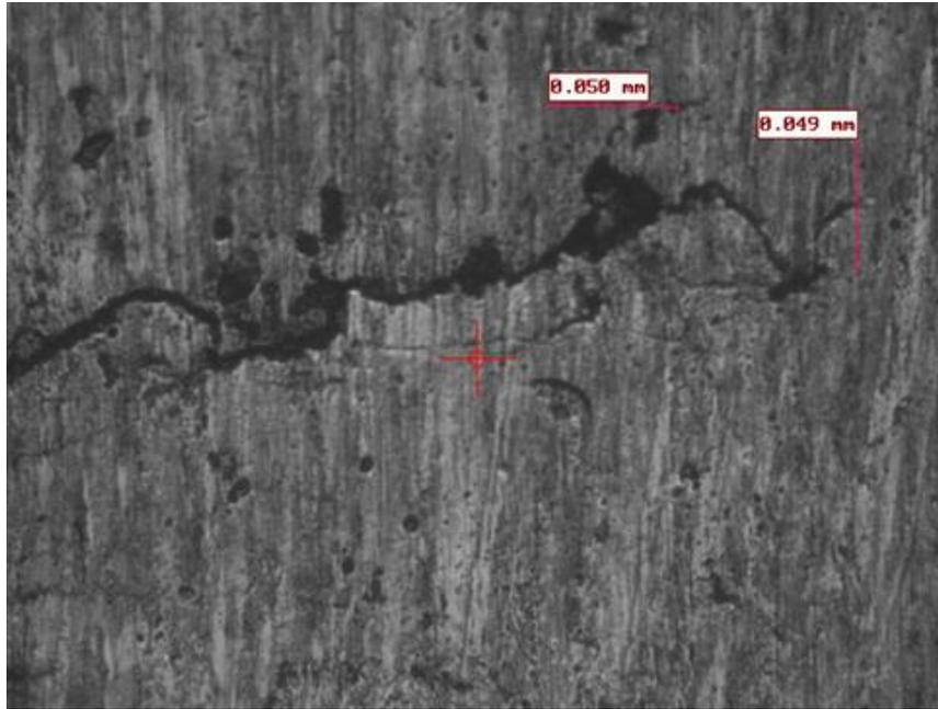
Figure 0.19: RCF-1-15, 38.5% Increased Contact Width, crack 1.3mm
