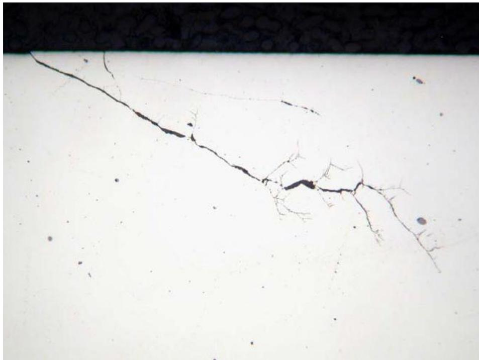
Figure 5.18: RCF-5-09, Crack Location Unetched (201X)
