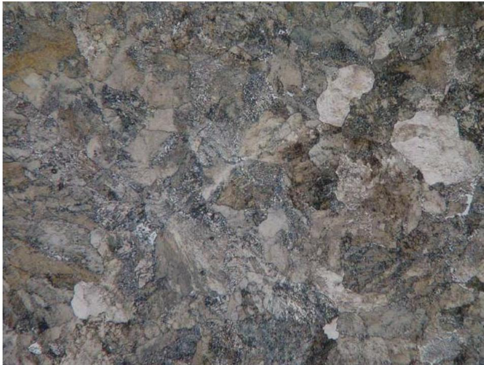
Figure 5.6: RCF-1-07, Fine lamellar pearlite with small amounts of ferrite. (494X)
