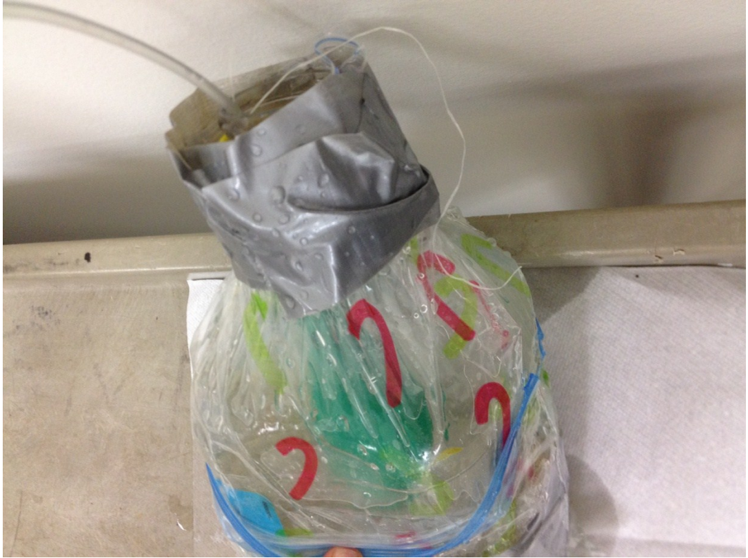
Top of the vessel used to house the balloon suspended in water.
