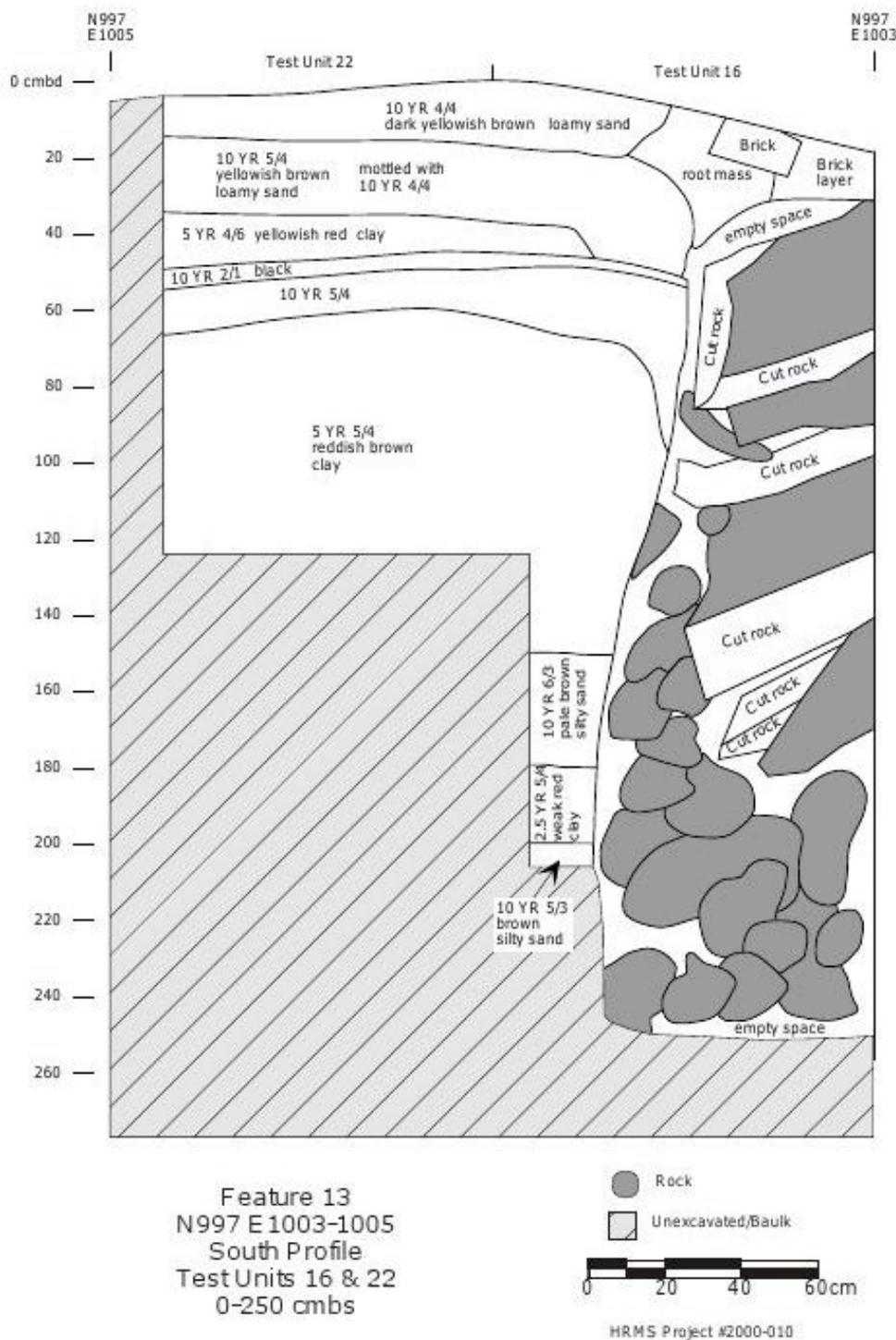
Figure 22: Feature 13 south profile in test units 16 and 22
