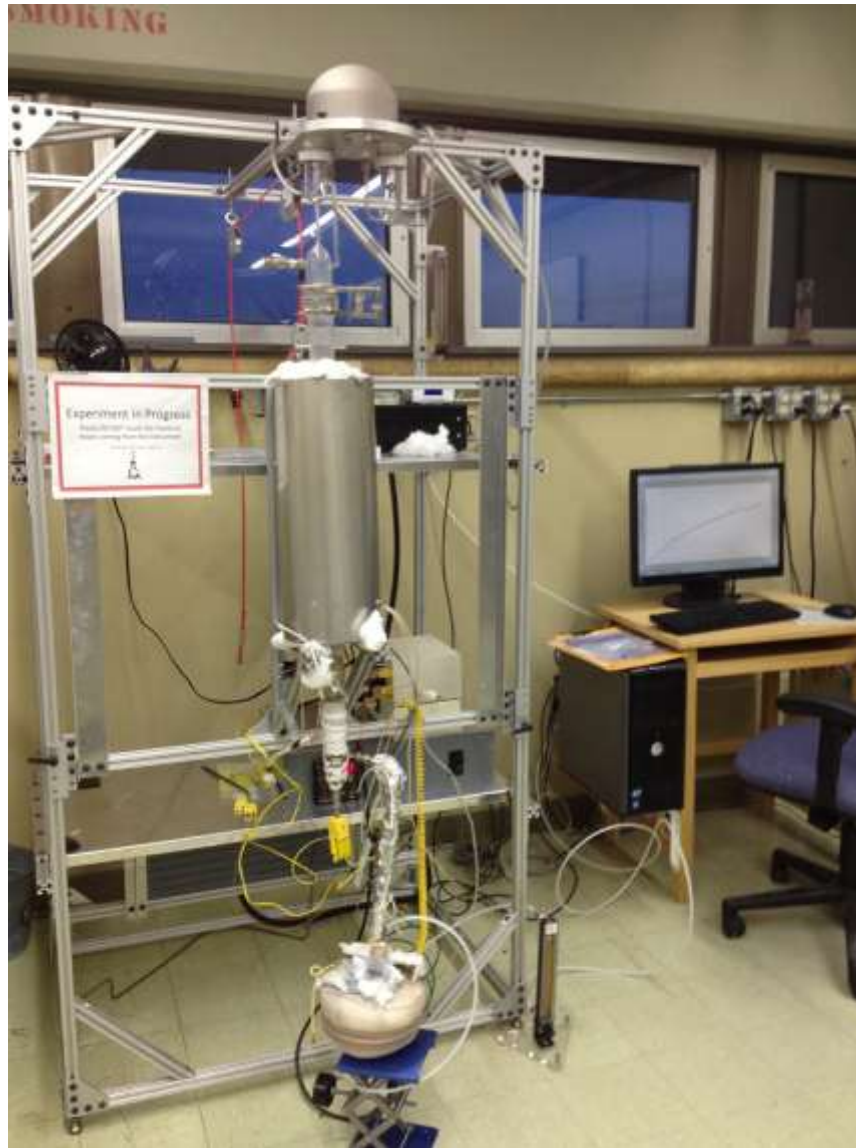
Figure 12. Custom built Thermogravimetric Analysis Equipment
