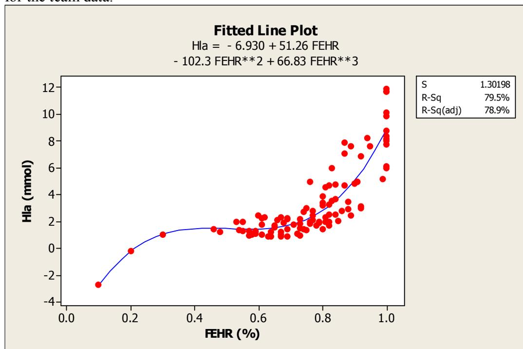
**Figure D-2:** Fitted line plot of the Hla vs. FEHR using a 3<sup>rd</sup> degree polynomial extended to smaller values of the FEHR for the team data.
