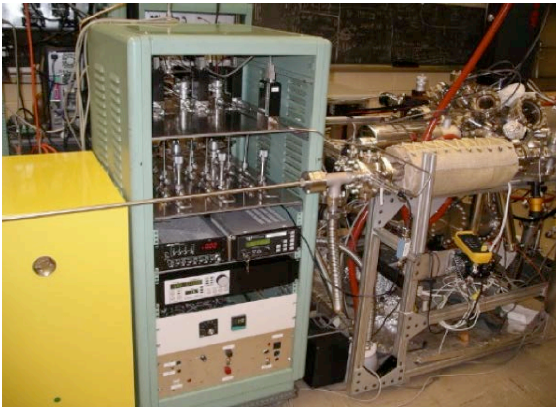
Figure 3.13 Viscous-flow UHV-interfaced ALD reactor with in-situ QCM.
