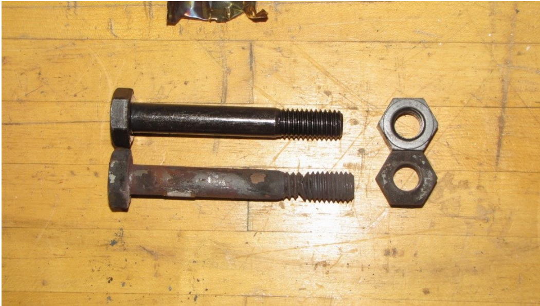
Figure 3-13 A comparison between the bolt before and after the test
