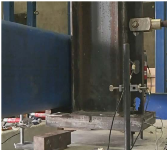
Figure 2.38 Two-bolt compression and shear test. A) Fully instrumented specimen. B) Plan view detail of base plate. (Photo from McBride (2019))
