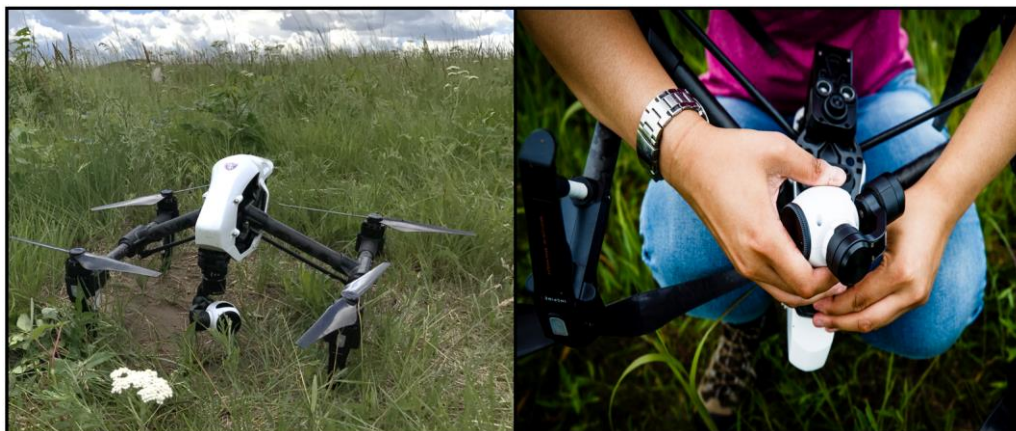
Figure 3. The DJI Inspire 1 quadcopter, used for this project. On the right: a close-up of the standard Zennuse X3 camera.
