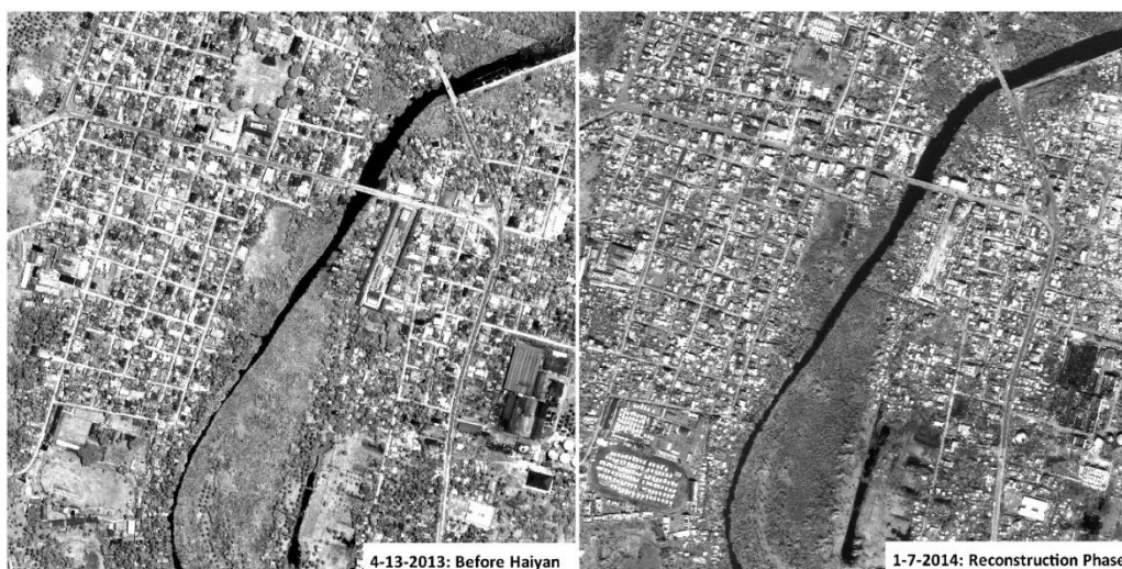
Figure 5. Remote Sensing analysis of the municipality of Tanauan (Leyte, Philippines) before and after Typhoon Haiyan to assess disaster damage and recovery using Geoeye and WordView VHR satellite imagery. In January 2014 large parts of the municipality are uninhabitable. Machine learning algorithms can be used to train for the detection of structural features such as temporary shelters (lower left corner). (Source: Authors' own draft)
