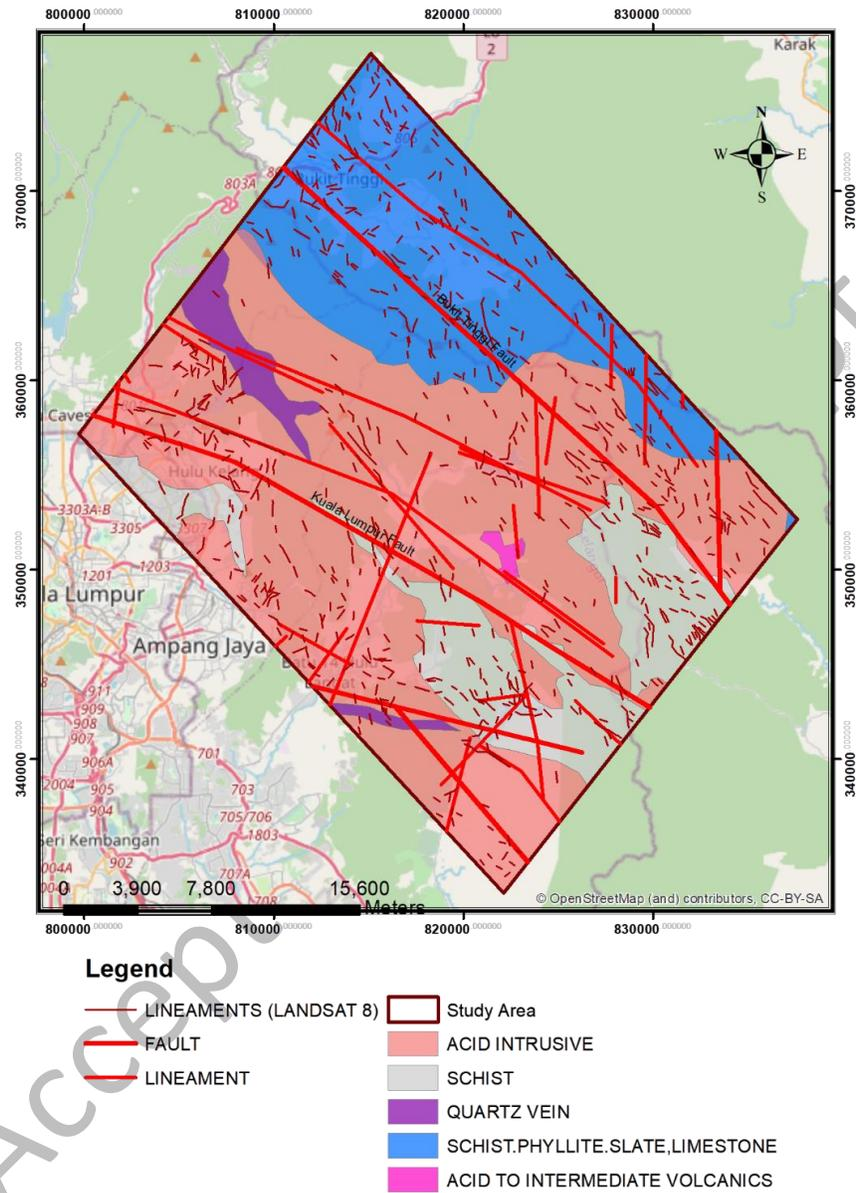
Figure 8. Overlay of the extracted lineaments from Landsat 8 to the geological map.
