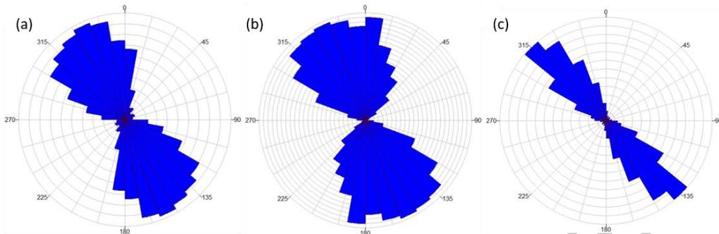
Figure 6. Rose diagrams of lineament extracted from Landsat 8 (a), Sentinel 1 (b), and Sentinel 2 (c) sensors, respectively.
