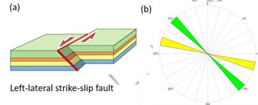
Figure 7. (a) Illustration of sinistral or left-lateral strike-slip fault where the left block moves toward and the right block moves away (Butler et al., 2009) and (b) Trending of Bukit Tinggi fault (green) and Kuala Lumpur fault (yellow) in a rose diagram.
