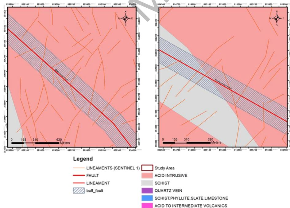
Figure 12. Example of matching and non-matching lineaments near Bukit Tinggi Fault Zone (left) and Kuala Lumpur Fault Zone (right)
