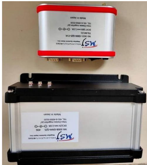
Figure 2. Albicila Version (upper) and Luscinia 2+ Version (lower) of MSJ's receivers used in this study.
