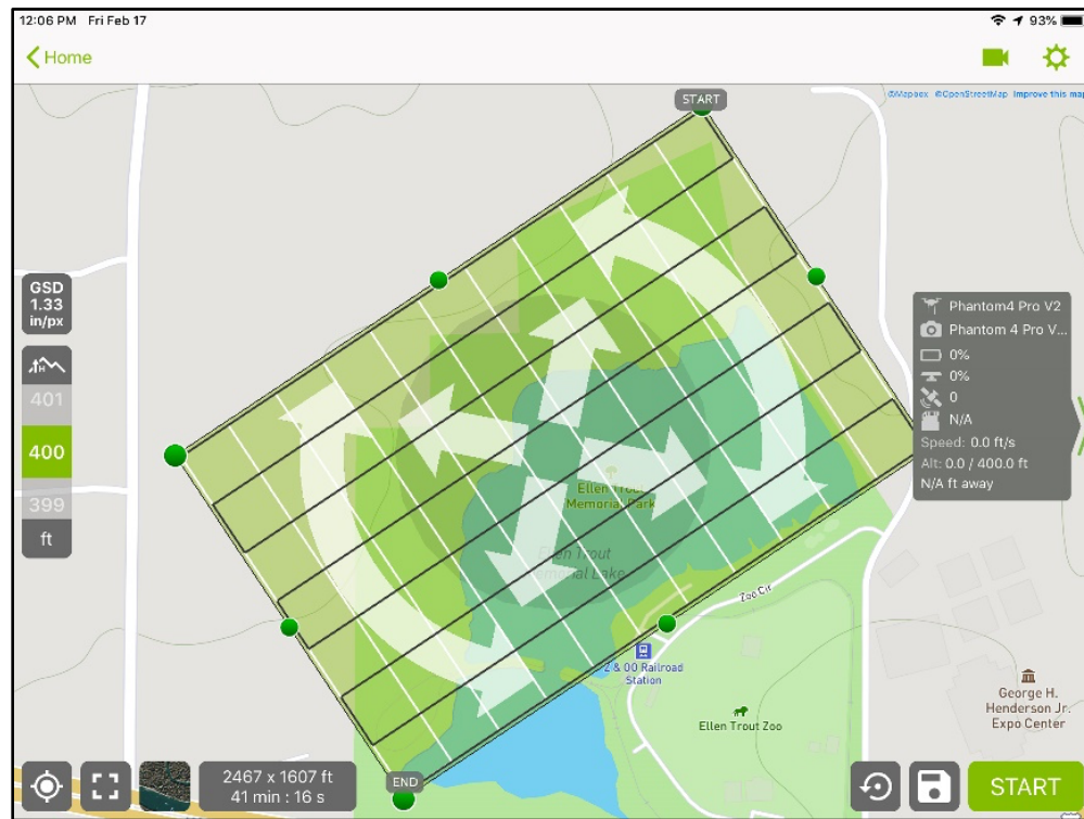
Figure 5. Double pass drone flight configuration designed in Pix4Dcapture.
