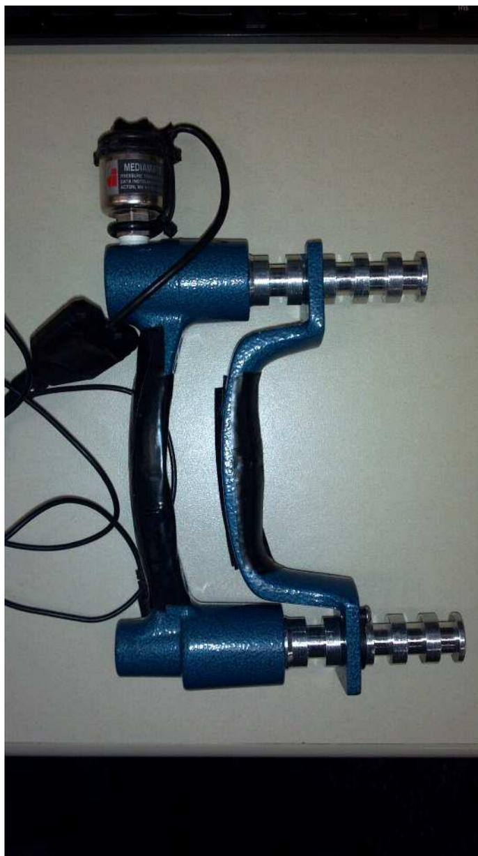
**Figure 3.1 Jamar Dynamometer**
