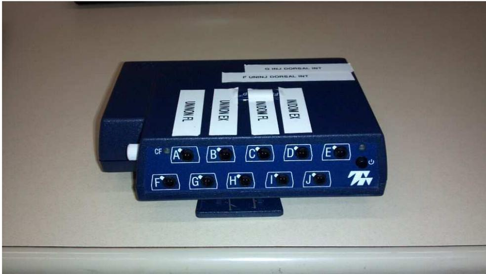
**Figure 3.2 FlexComp Infiniti Analog to Digital Converter**
