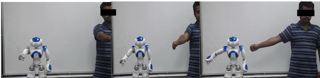
Figure 5.9 Arm position of human operator and NAO robot during Shoulder joint horizontal flexion/extension motion during teleoperation
