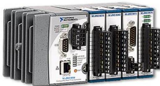
**Figure 6-15 System controller (CompactRIO) from national instruments.**
