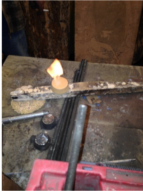
Figure 4: The top of a sand core that has been ignited with a blowtorch.
