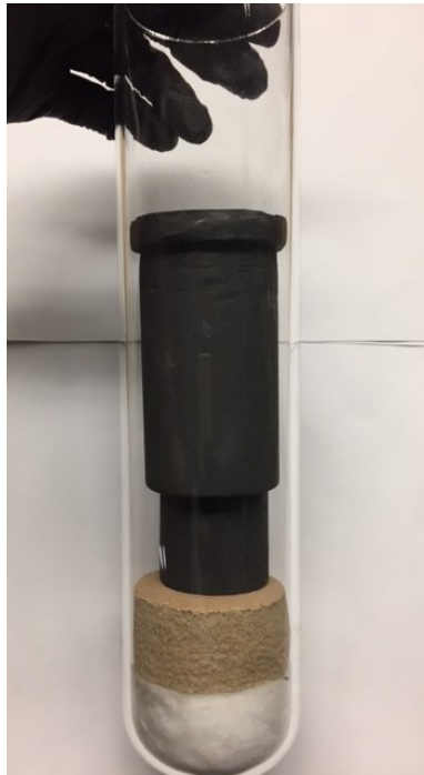
Figure 10: The quartz tube with all of the components used for casting in a small induction furnace.
