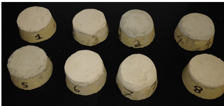
Figure 5: Eight cores with alloying element-containing slurry hardened on top of them. The tops of the cores had been smoothed with sandpaper.
