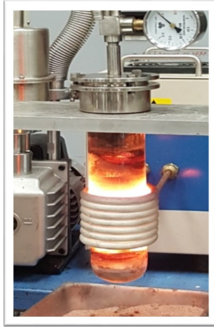
Figure 11: The red-hot quartz tube on the vacuum pump as the steel is being melted.
