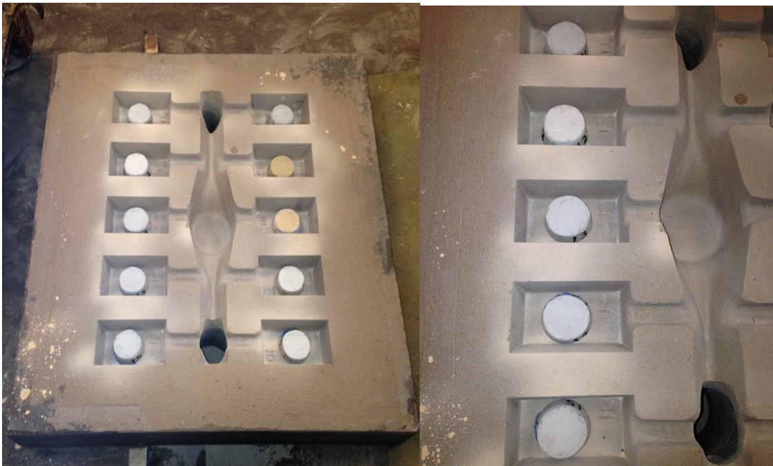
Figure 7: The drag side of the sand mold with the sand cores placed inside the test cavities. The mold was then closed, and steel was cast into it.
