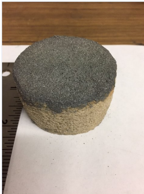
Figure 17: The dried on nickel and chromium slurry prior to delivery to Maynard Steel.
