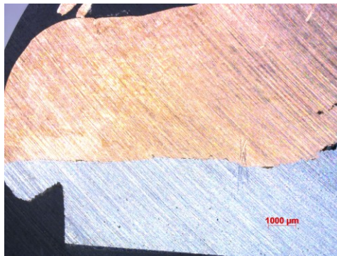
Figure 15: The mounted sample of copper and steel made by induction melting in the UWM foundry lab.
