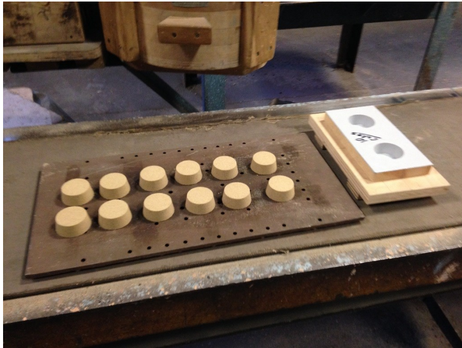
Figure 3: Core box and 8 uncoated sand cores provided by Maynard Steel
