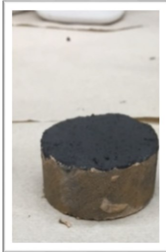
Figure 14: The slurry-coated core still wet before drying in a low-temperature furnace.
