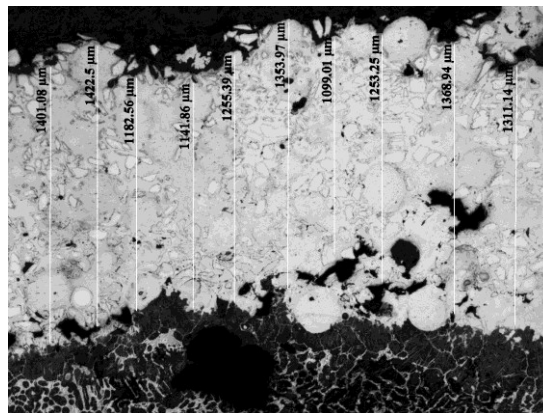
Figure 22: The microstructure the surface and substrate of UWM Sample #3.
