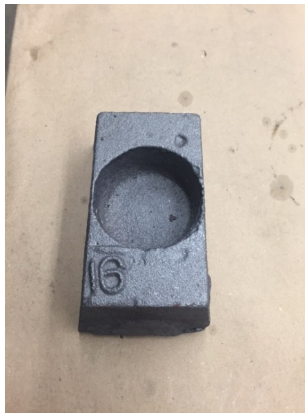
Figure 8: The ten-pound test block. The enriched surface is the one that came in contact to the slurry, which is the flat, recessed surface that is visible.
