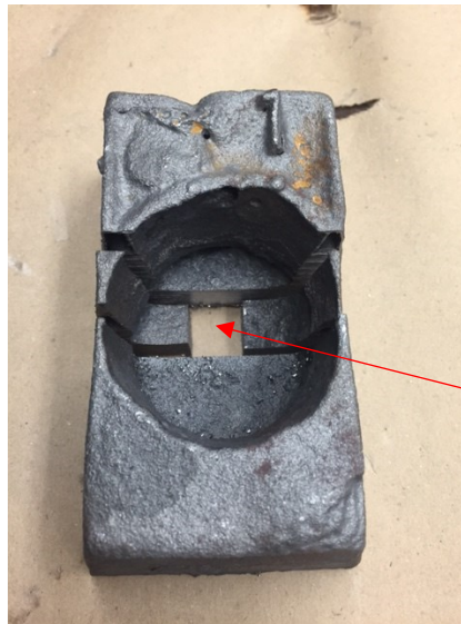
Figure 9: The center cube was cut out from the test block. This sample was mounted in such a way that the cross-section from the surface into the substrate could be studied.
