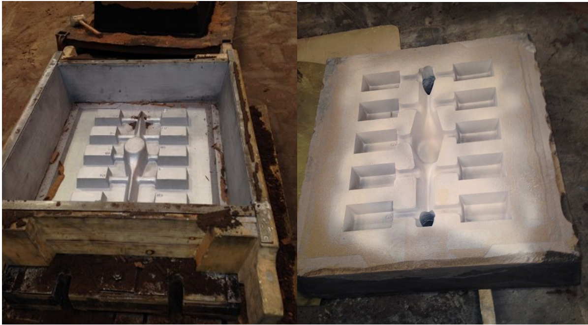
Figure 6: The cope and drag of the sand molds in which the cores were placed.
