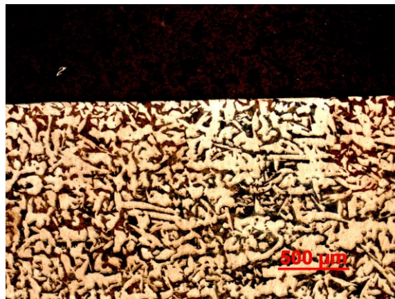
Figure 19: The surface of UWM Sample #1 showing pearlite and ferrite in the microstructure, although no surface layer is evident.
