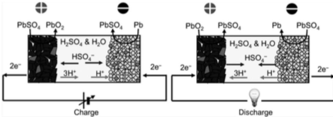
**Figure 10. Principles of operation of a lead-acid battery**
