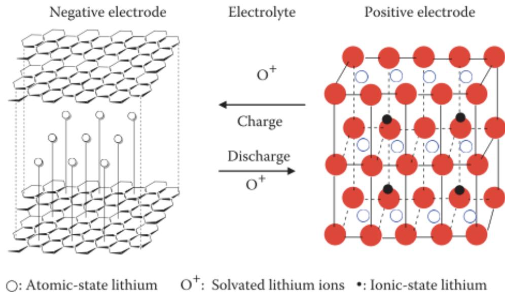
**Figure 9. Principle of operation of the lithium-ion battery**
