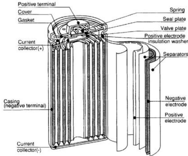
**Figure 8. Structure of a cylindrical NiMH battery**
