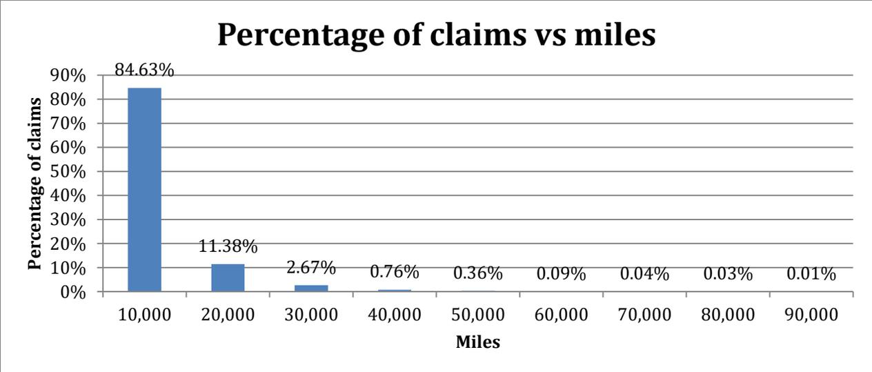
**Figure 18. Percentage of claims versus miles until failure**
