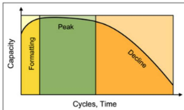
**Figure 1. Three main phases of the lifespan of a lead acid battery.**
