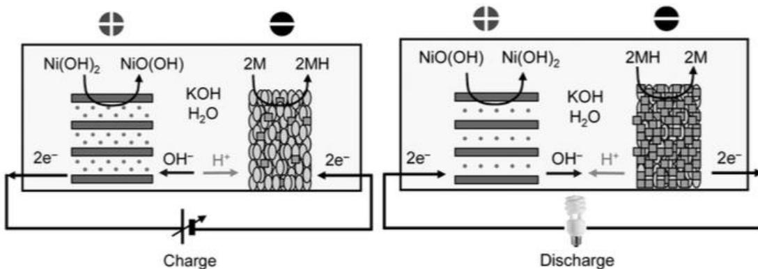
**Figure 7. Reaction principles of NiMH batteries**
