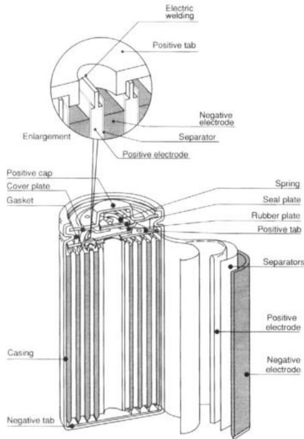
**Figure 6. Structural design of a cylindrical portable nickel-cadmium**
