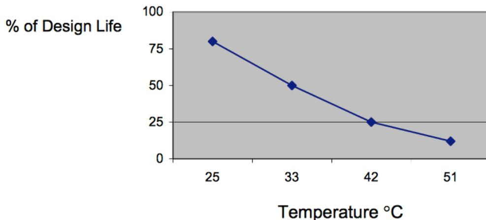
**Figure 2. Battery design life vs. environment temperature**
