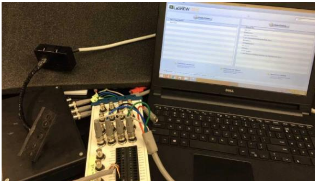
Figure 2.2 Cytometer system consists of DAQ board, control box, computer LabVIEW software and probe.
