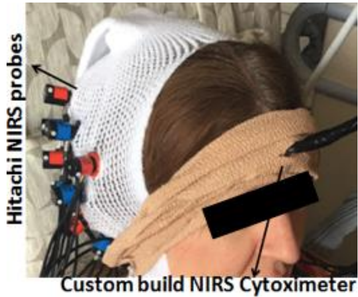
Figure 3.3 Epilepsy protocol, NIRS Cytosimeter is attached at forehead of the subject and Hitachi NIRS probes are attached at back of the head.
