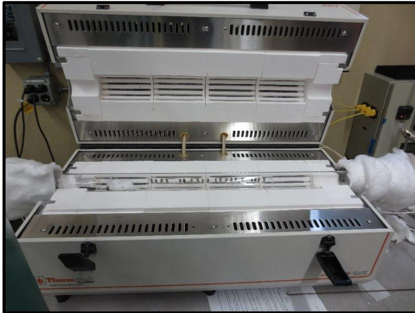
Figure 12. Illustration of the specimens put in the oxidation apparatus
