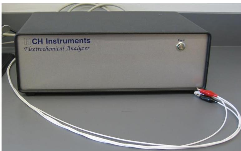
Figure 5: CHI-6012E, a computer-controlled electrochemical analyzer (CHI, USA)
