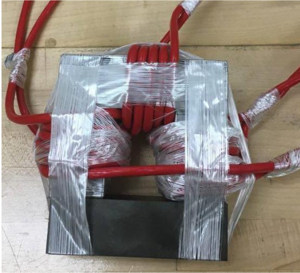
Figure 5-11. Final assembled multi-winding HF transformer
