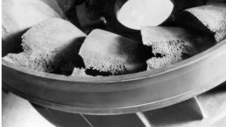
Figure 2: Cavitation damage on the blades at the discharge from a Francis turbine [9]
