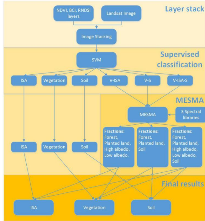
Figure 13 Flowchart of class-based MESMA. High albedo, low albedo, and ISA were combined as ISA. Forest, planted land, and vegetation were combined as vegetation. Soil in soil pure land cover class and soil in fraction images were combined as soil.
