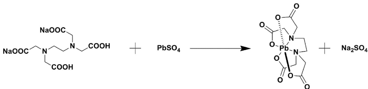
Figure 10: Chelating additive Na 2 EDTA mechanism with lead sulfate. [52]
