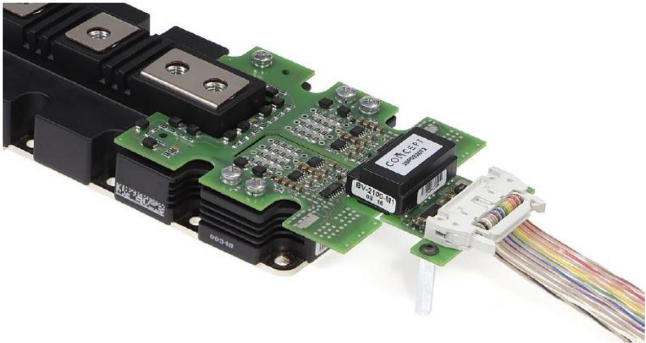
Figure 4.29 Gate drive, IGBT and X1 connector [11]
