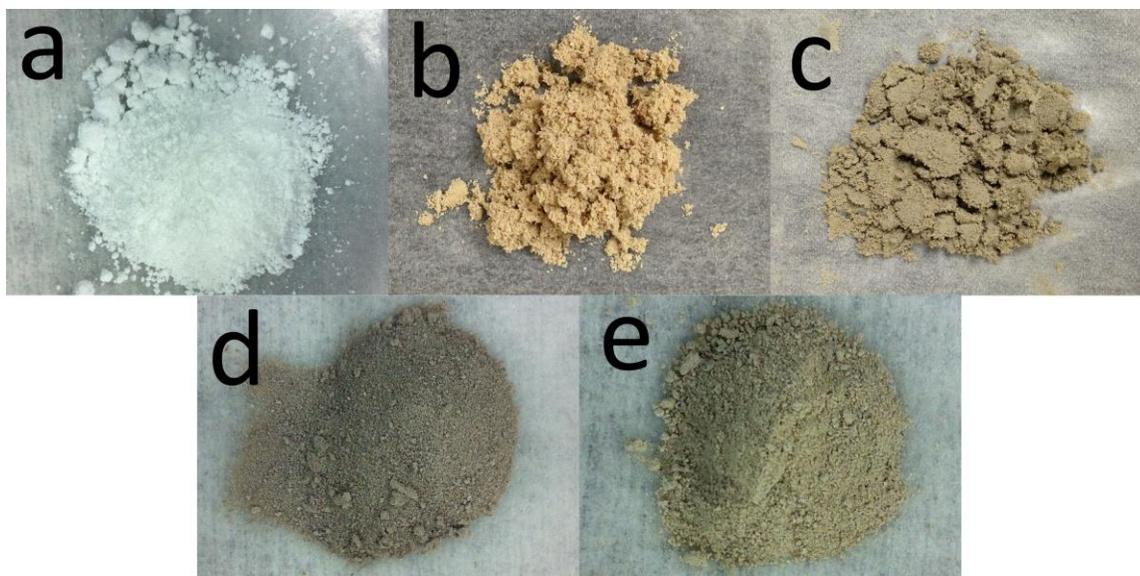
Fig. 2.1 Photographs of pristine TiO<sub>2</sub> (a) and doped TiO<sub>2</sub> samples, (b) TiO<sub>2</sub>-1, (c) TiO<sub>2</sub>-2, (d) TiO<sub>2</sub>-3 and (e) TiO<sub>2</sub>-4.
