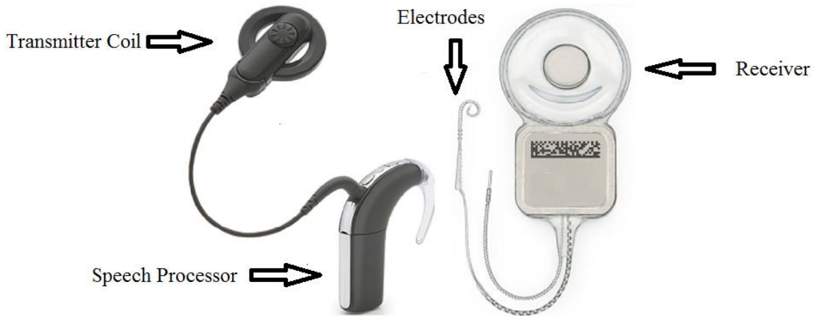
Figure 1-3 Structure of cochlear implant
