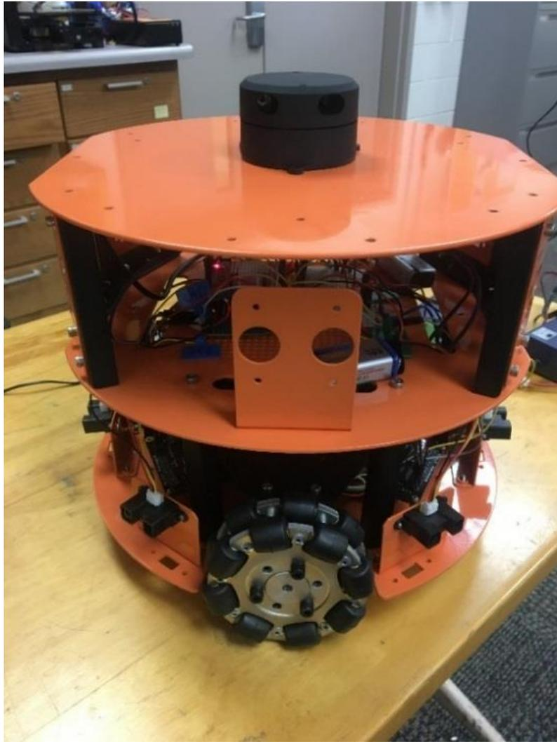
**Figure 7:** HCR Omni wheeled robot with LIDAR
