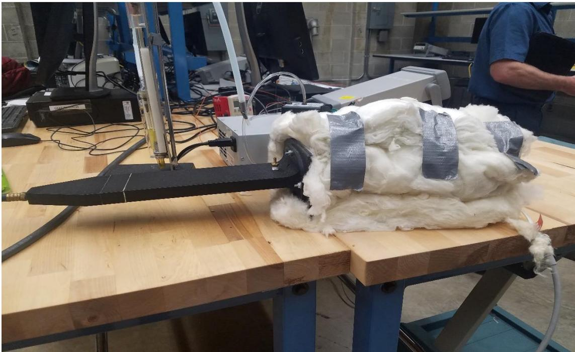
**Figure 7.24** Final setup using fiberglass wool insulation.
