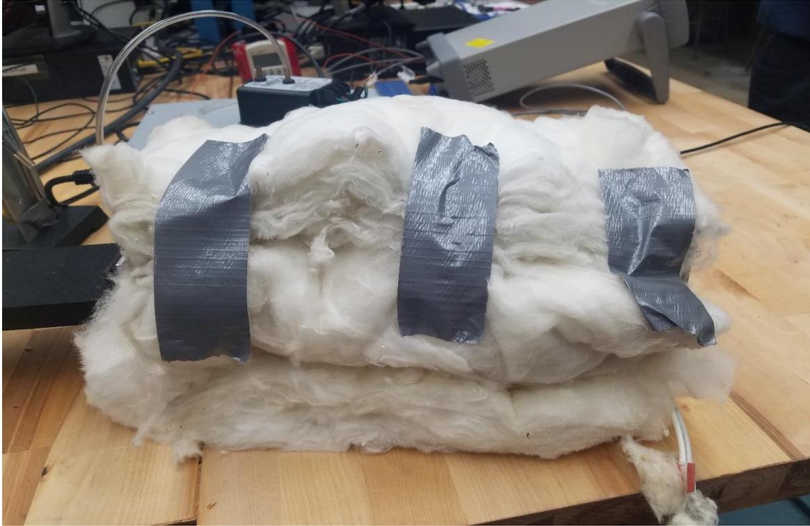
**Figure 7.25** Fiberglass insulation around the fin assembly.
