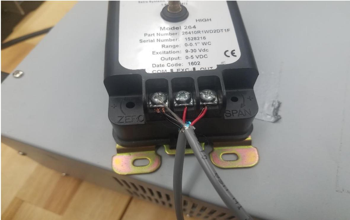
**Figure 7.20** Pressure transducer connection.
