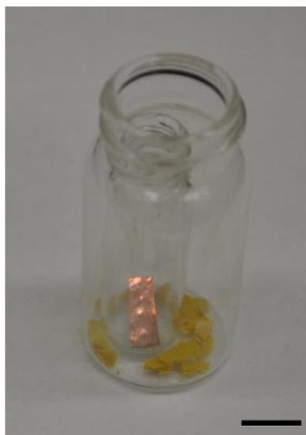
**Figure 2.1.** Photo of the reaction setup before sealing and injection of dilute H<sub>2</sub>SO<sub>4</sub> solution. The double vials ensure that the graphene sample is only exposed to H<sub>2</sub>S gas which is generated *in situ*, not any liquids or solids. Scale bar: 1 cm.
