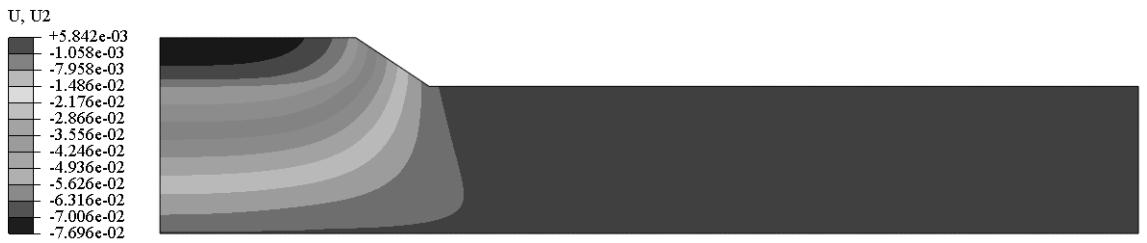
Figure 5.23 Vertical deformation contour of analysis No.6 ( ft )
