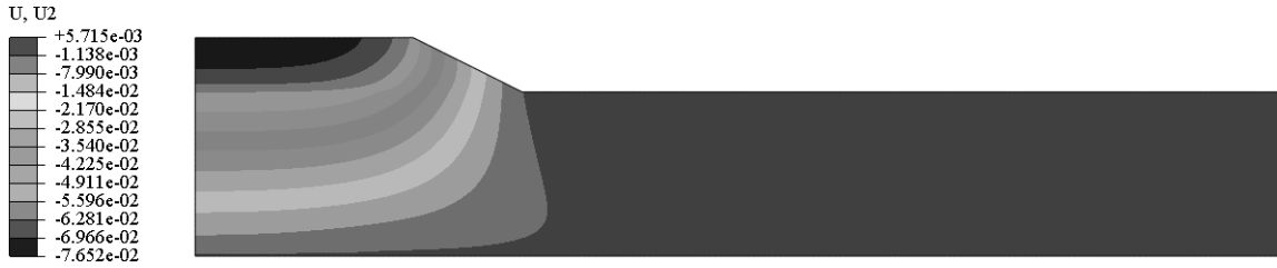
Figure 5.20 Vertical deformation contour of analysis No.3 ( ft )
