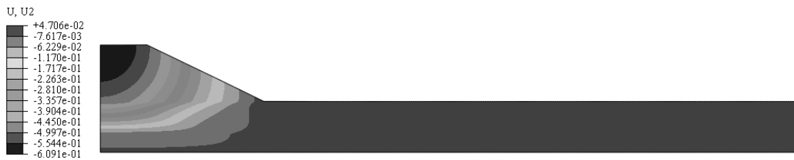
Figure 5.13 Vertical deformation contour at the end of the analysis ( ft )
