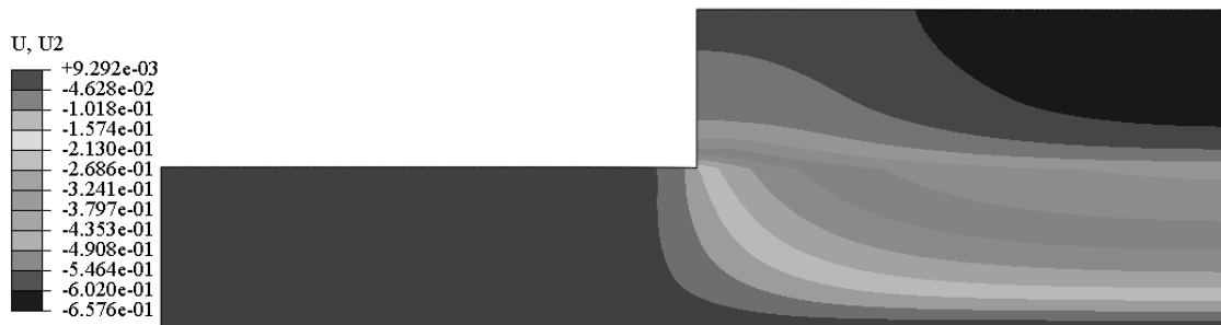
Figure 5.82 Vertical deformation contour (transverse direction) of soil profile No.1 with additional fill ( ft )
