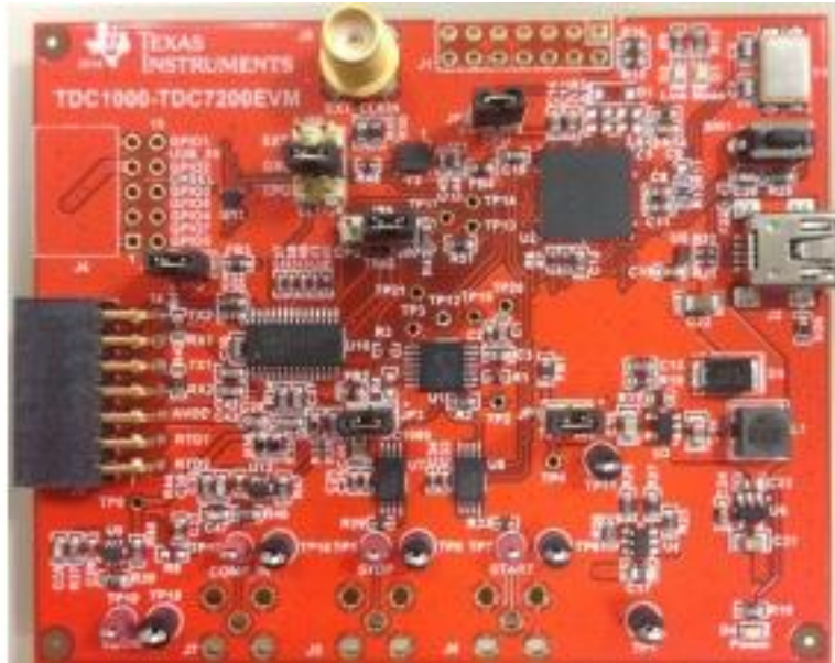
Figure 2.3: TDC1000 - TDC7200 EVM Evaluation board (Source: ti.com).
