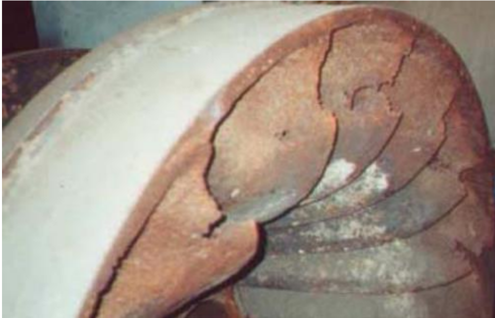
Figure 2-13: Severe cavitation erosion effect on Francis runner blades[68]
