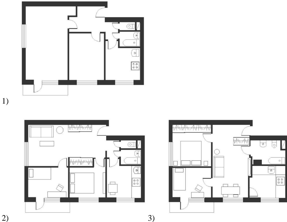
Fig.3.7. 1) A plan of a two-room apartment (I-515/5 series) before remodeling and re-planning; 2) and 3) plans of the same apartment re-planned to have two isolated bedrooms and a separate living room space.<sup>70</sup> Both of these re-planning options indicate a separation between night time and date time spaces. Both suggest direct access to each bedroom from a communal space.
