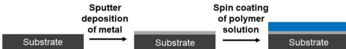
**Figure 3.3.** Schematic illustration of the preparation of the thin films of polymer on metal-coated substrates.
