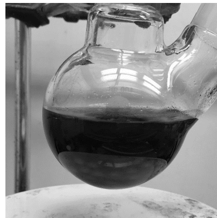
Figure 14: Finely ground, oxidized PDC turning black during the reaction
