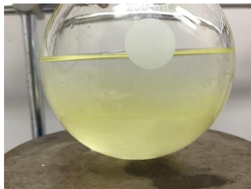
Figure 12: Faintly seen aqueous and organic layers as reaction turns yellow in Pinnick oxidation
