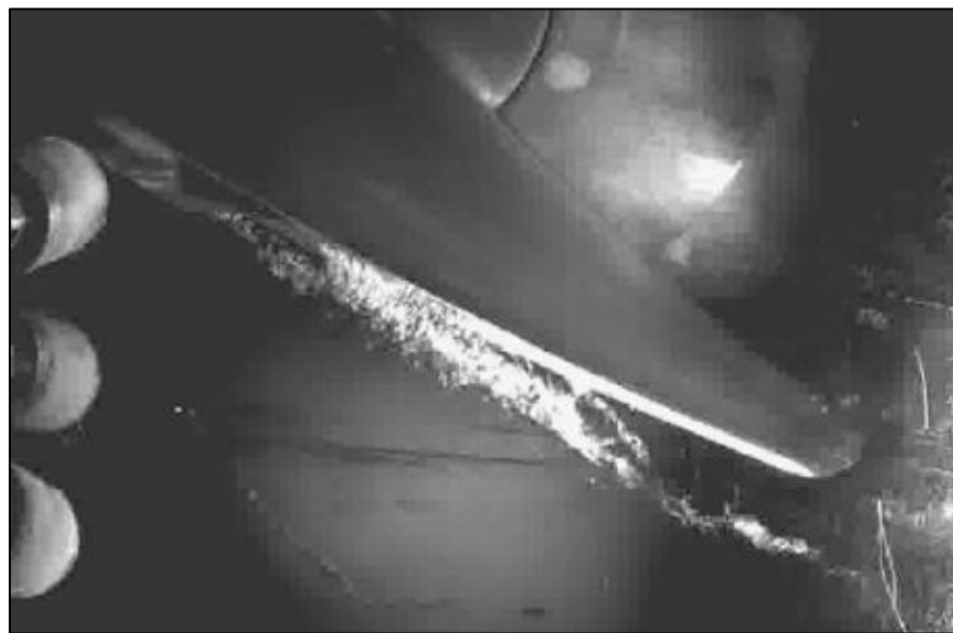
Figure 6: Tip vortex cavitation as witnessed on a Kaplan runner [12]
