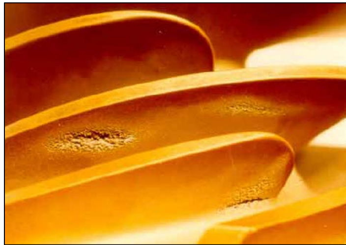
Figure 4: Localized cavitation damage on a pump blade [9]
