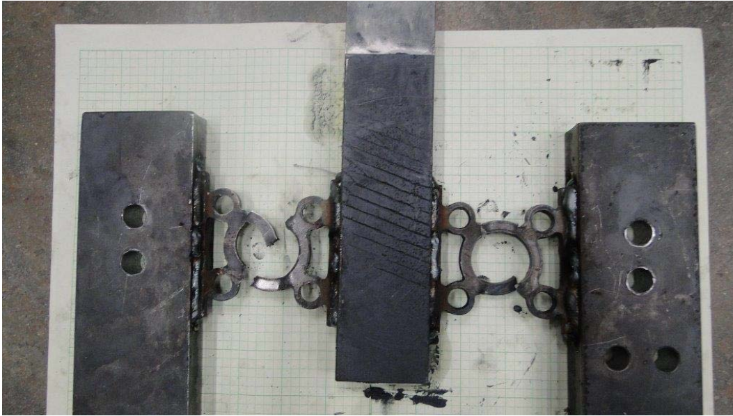
Figure A- 13: Failure mode of third set of tested devices
