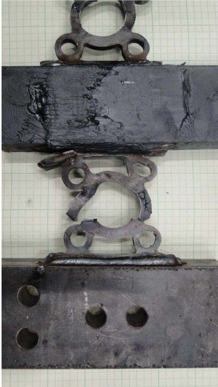
Figure A- 7: Close-up of the fist tested device shows the failure mode
