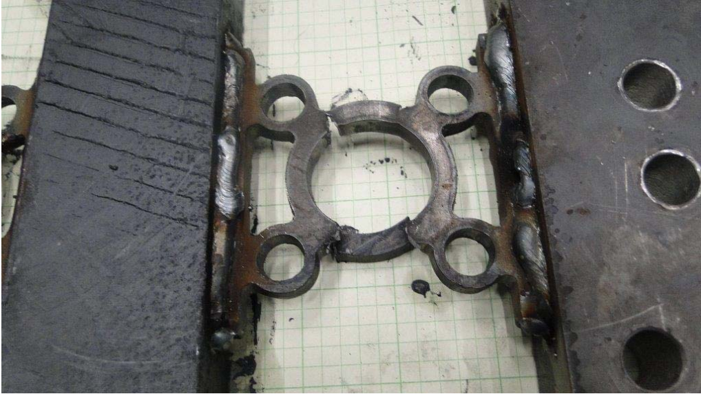
Figure A- 15: Close-up of the third set of tested device shows the failure mode
