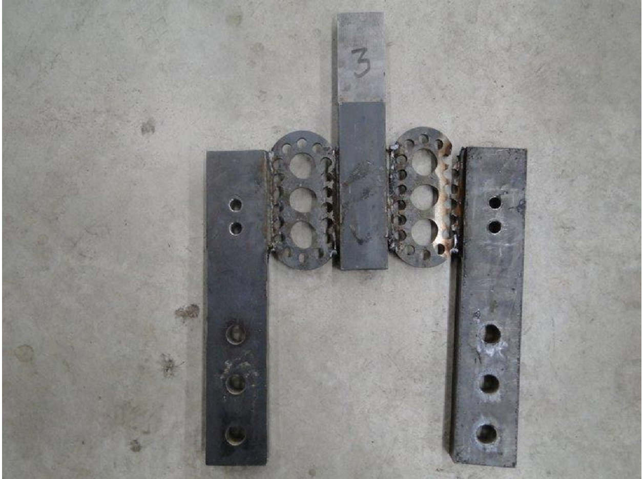
Figure A- 24: Failure mode of third set of tested NS-5 shapes
