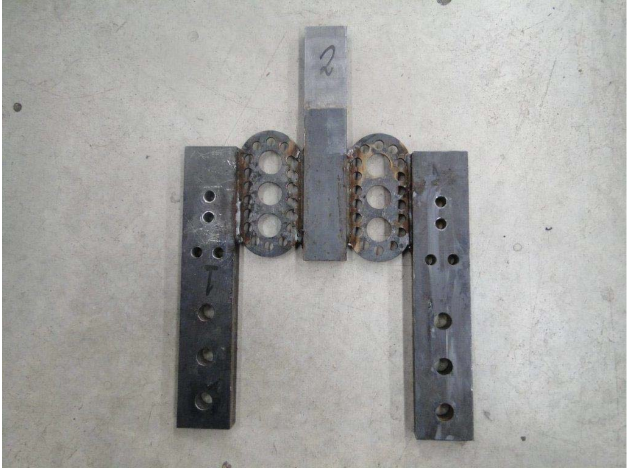
Figure A- 21: Failure mode of second set of tested NS-5 shapes
