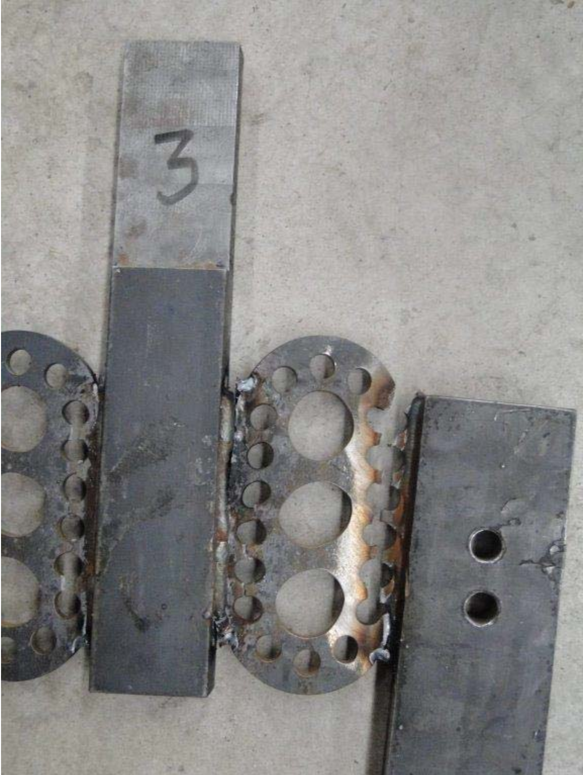
Figure A- 26: Close-up figure shows the failure initiation of third set of NS-5 shapes
