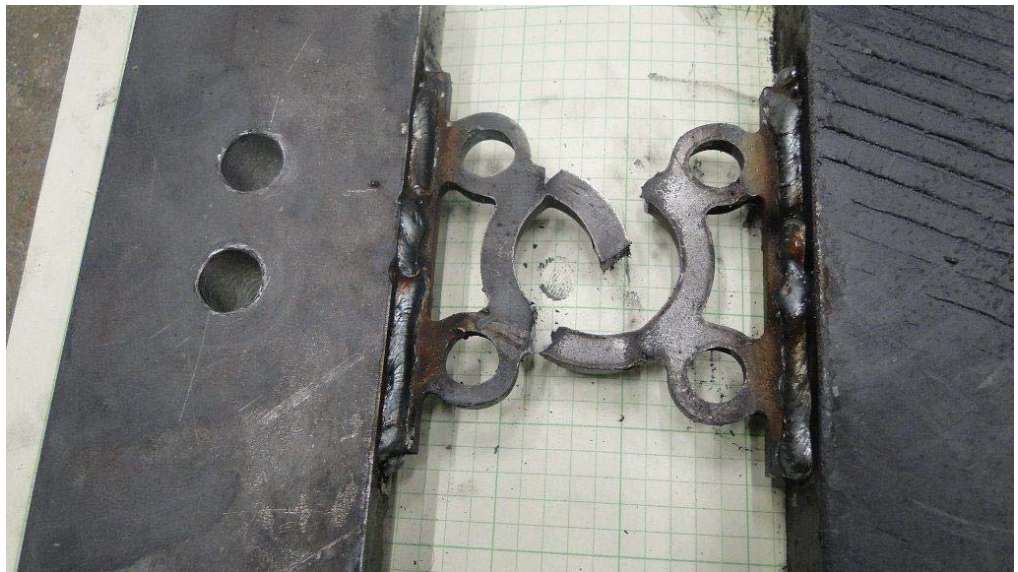
Figure A- 16: Close-up of the third set of tested device shows the failure mode
