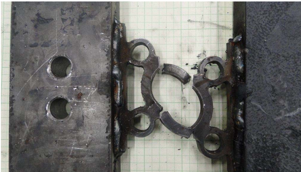
Figure A- 12: Close-up of the second tested device shows the failure mode
