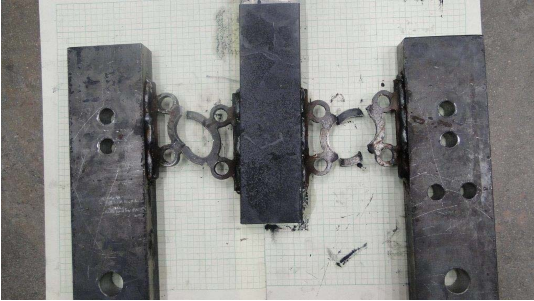
Figure A- 9: Failure mode of second tested devices
