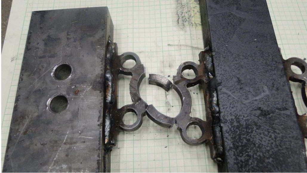
Figure A- 11: Close-up of the second tested device shows the failure mode
