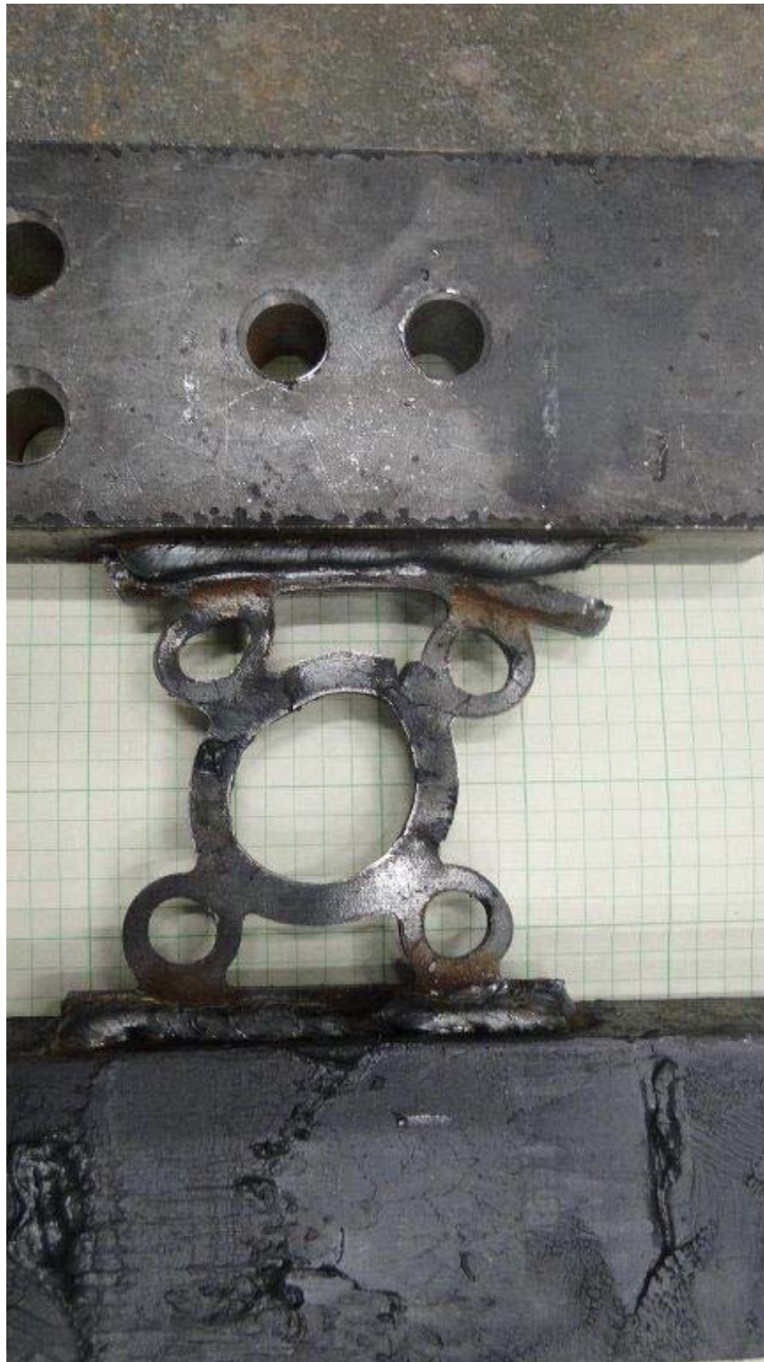
Figure A- 8: Close-up of the fist tested device shows the failure mode
