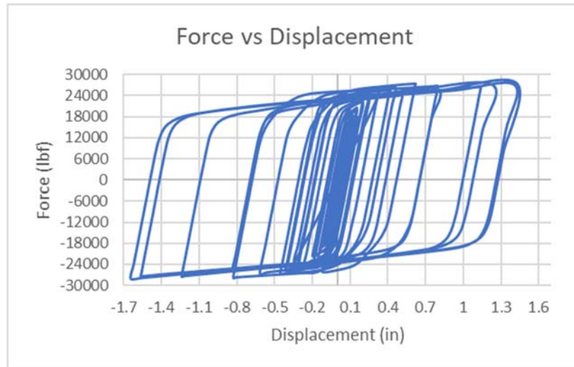
Figure 3-22: Finite elements results of U-shaped connector.
