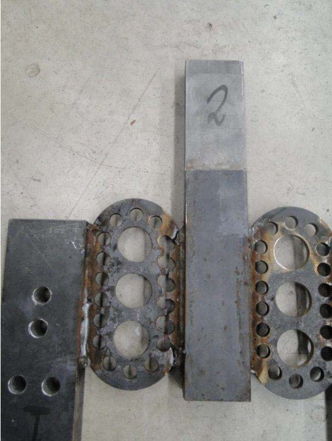
Figure A- 23: Close-up figure shows the failure initiation of second set of NS-5 shapes
