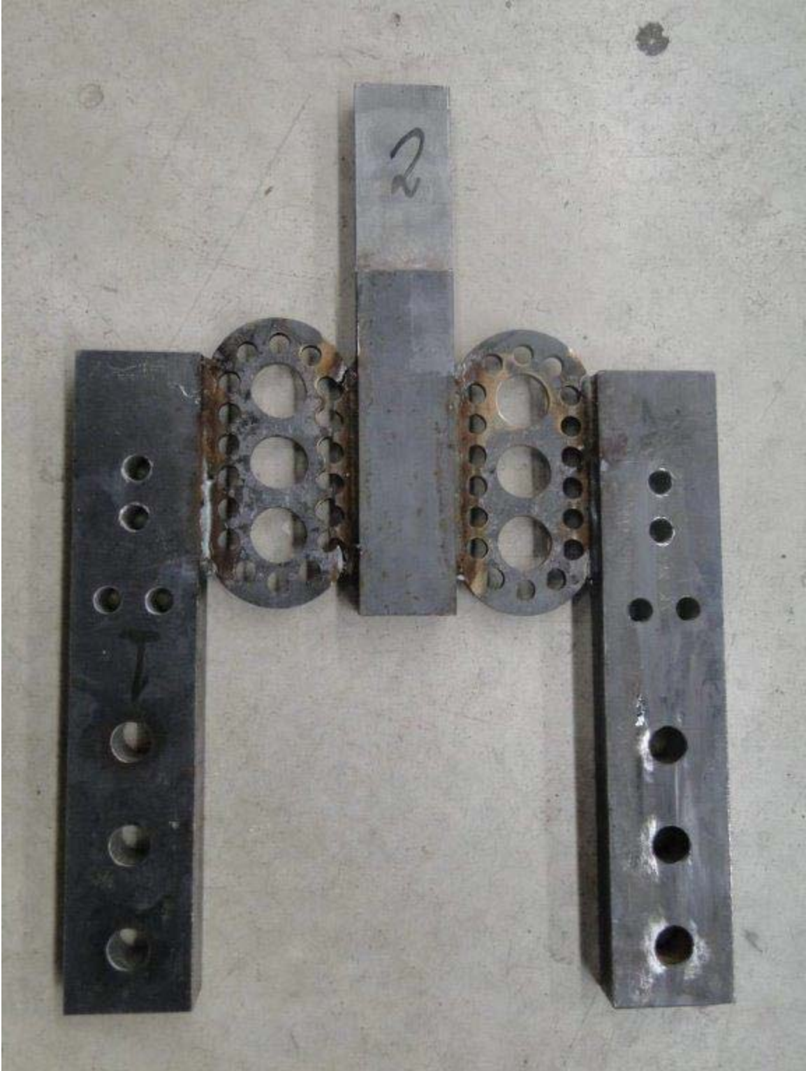
Figure A- 22: Failure mode of second set of tested NS-5 shapes shows the failure mode
