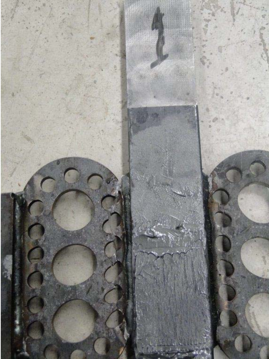
Figure A- 20: Close-up figure shows the failure initiation of first set of NS-5 shapes
