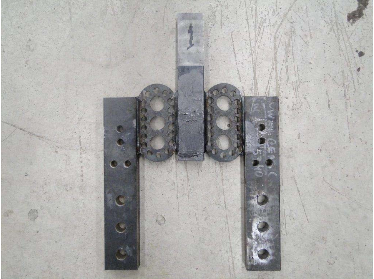
Figure A- 18: Failure mode of first set of tested NS-5 shapes
