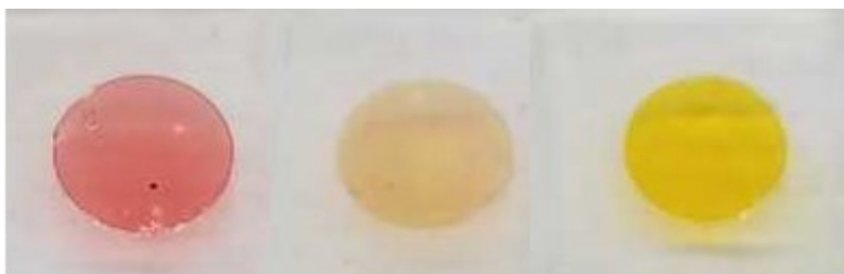
Figure 47. Examples of the final amino terminated hydrogel polymers loaded with PAR. The polymer after exposure to \text{Zn}^{2+} (Left), buffered at pH 7.2 MOPS (Middle), and in 1 M HCl solution (Right).
