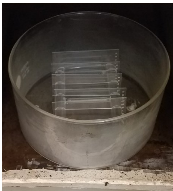
Figure 44. Setup to silanize up to 5 slides at a time.
