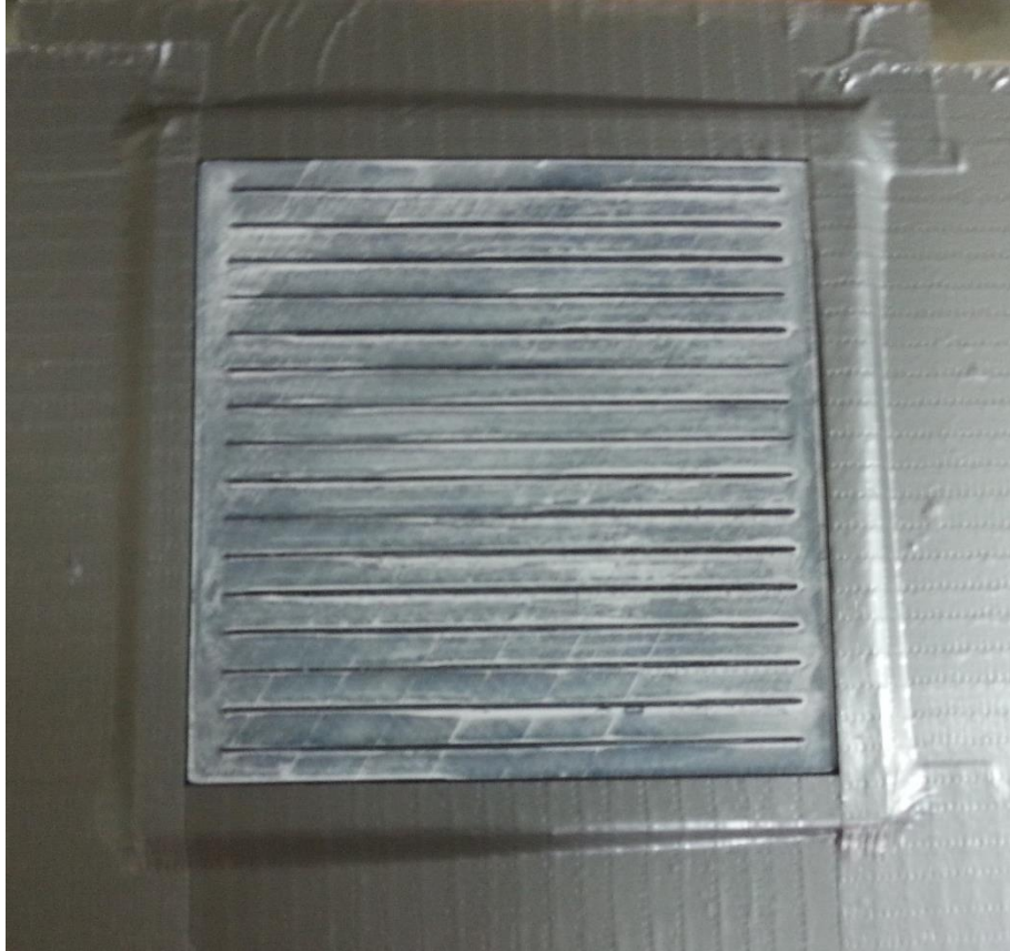
Figure 13: Self-contained 3D printed ABS template with paraffin wax coating.
