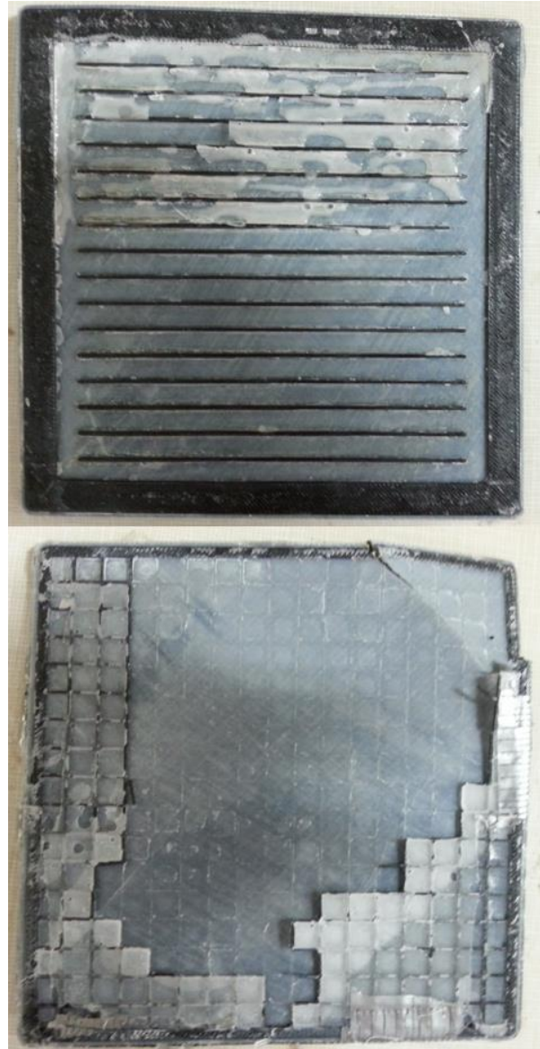
Figure 14: (Top) Vertical line template after FRP removal and (Bottom) Square grid template after FRP removal.
