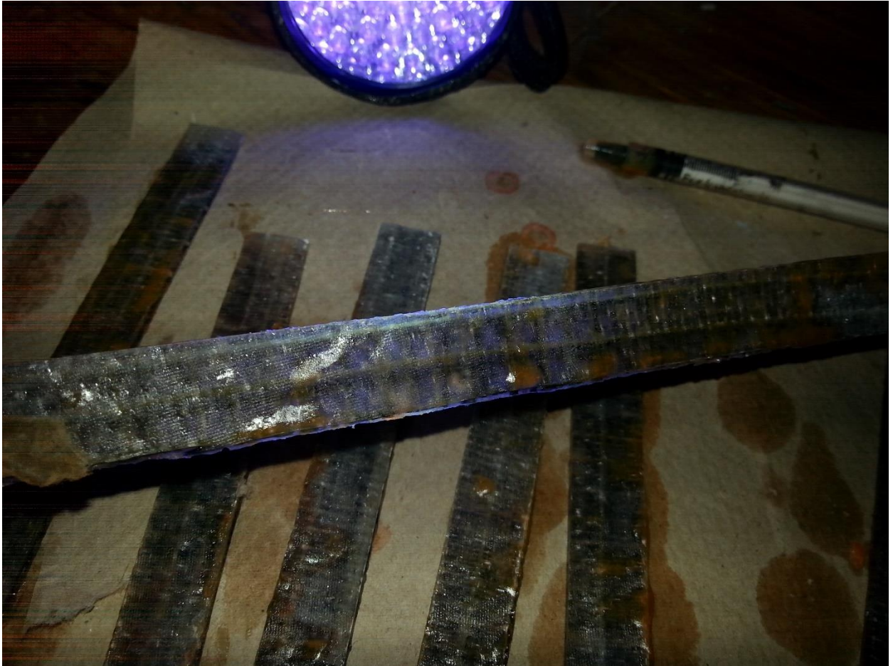
Figure 7: Wire formed network incorporated samples injected with DCPD.
