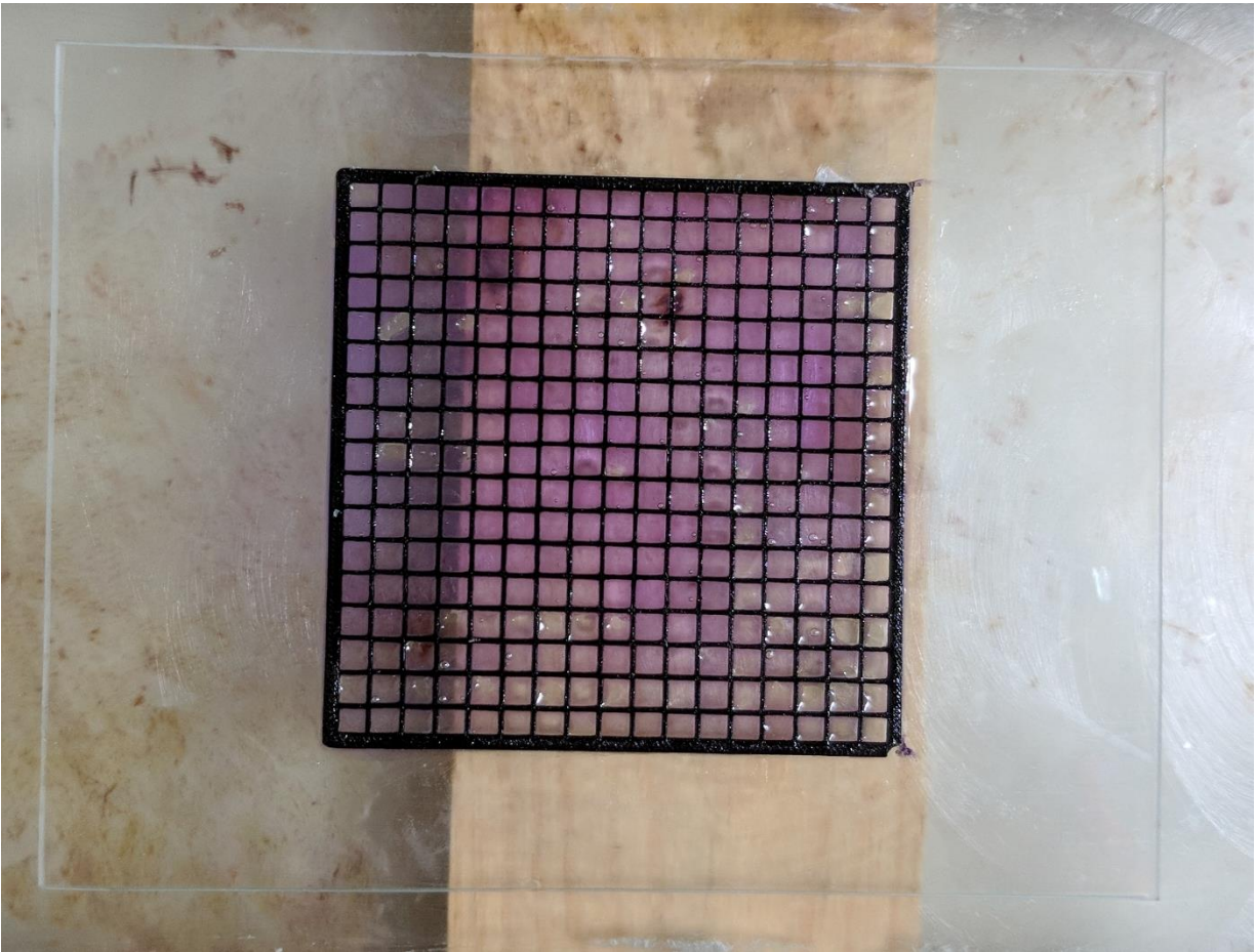
Figure 15: Square grid coated with water-soluble adhesive to aid in FRP removal.
