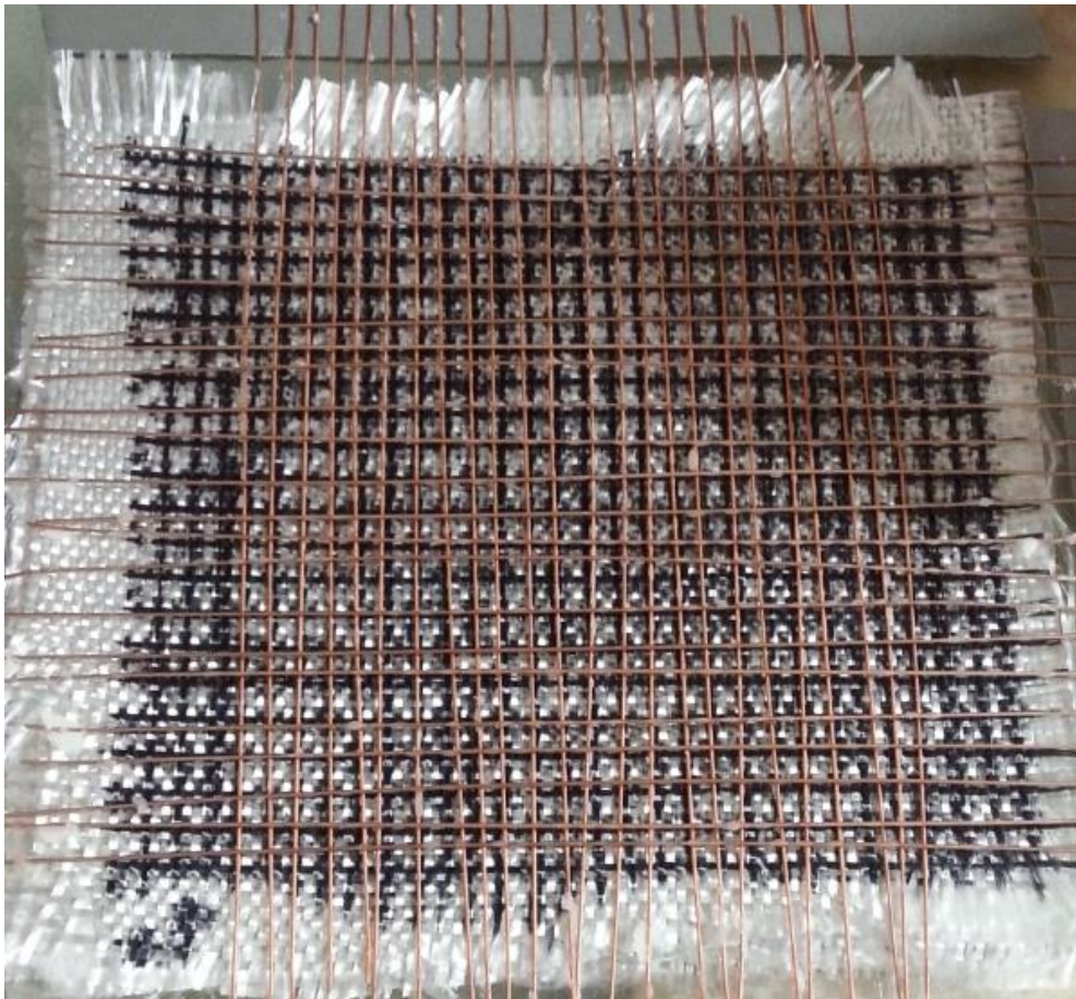
Figure 5: Uncoiled and straightened wire arranged in a grid configuration in the center layer of the sample with the ends of the wire extended past the perimeter of the glass fiber sheets to aid in removal.
