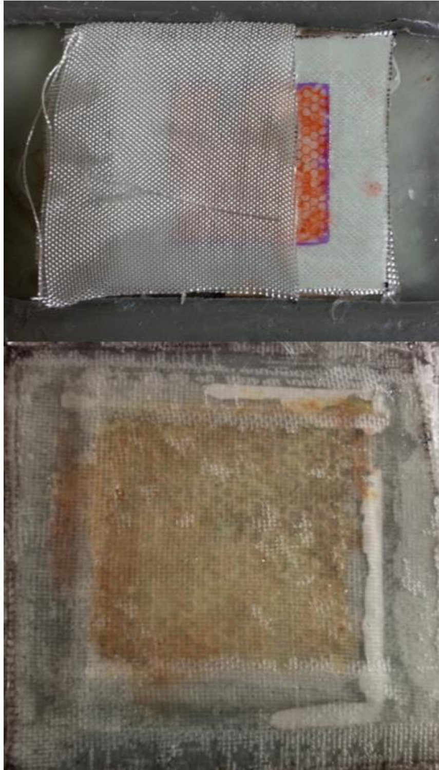
Figure 19: DCPD filled imprint layer placed in between fiberglass sheets. Before (Top) and after VARTM (Bottom)
