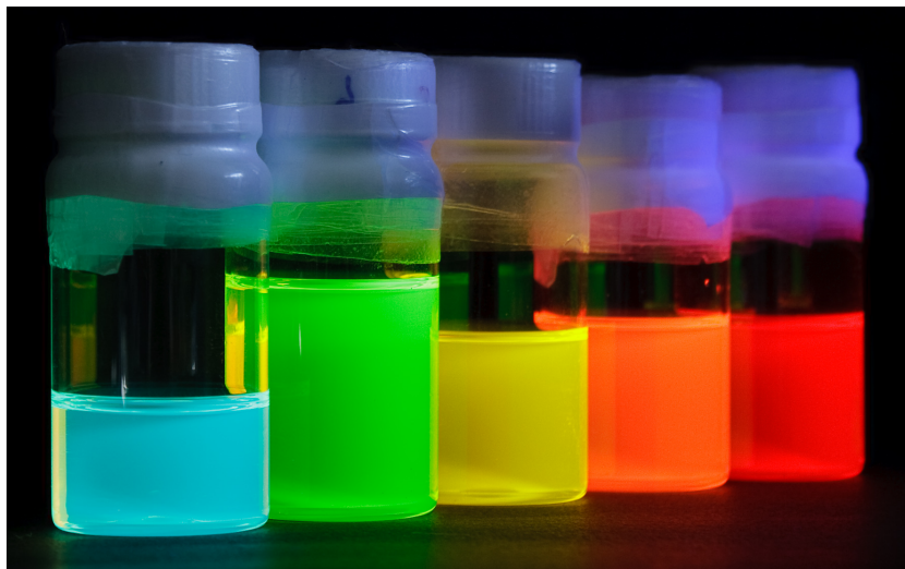
Figure 1-1: QDs of increasing size, from left to right, emitting cyan through red. QDs are dispersed in solution and illuminated by UV light source. 5
