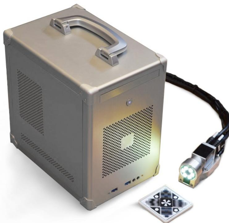
Figure 4: Single camera, single tracker system using Moiré Phase Tracking. The apparatus consists of a camera and reflective marker capable of rapidly and accurately collecting six degree of freedom data for each marker.
